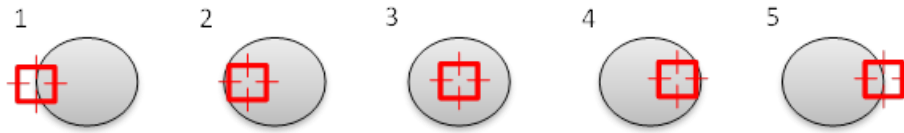
Figure 3.1 Five positions (1, edge-left; 2, area between edge-left and center; 3, center; 4, area between center and edge-right; and 5, edge-right) within one starch granule analyzed by Raman microspectroscopy.
