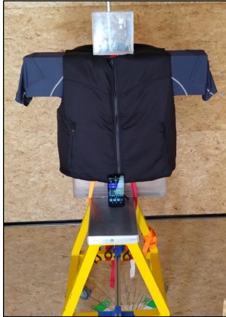
Fig. 6-21. Wireless WDD in prototype garment mounted on an ANSI 42.53 phantom.
