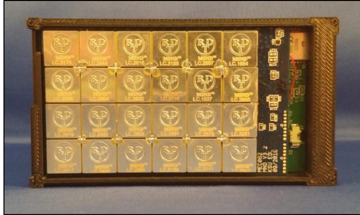
Fig. 6-6. Image of a wireless MND Mk III populated with 24, 1-cm 2 MSNDs with intrinsic thermal neutron detection efficiencies of 30%.
