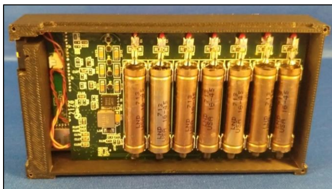
Fig. 6-20. Modular Gamma-ray Detector (MGD) with seven LND model 713 Geiger-Müller detectors. The wireless MGD has an onboard rechargeable battery, BLE communications board, and all required signal processing electronics.
