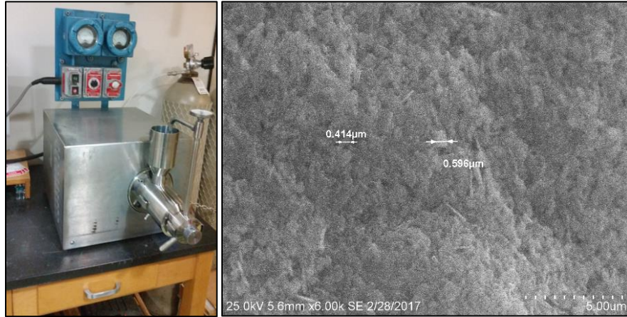
Fig. 5-16. (Left) Ball mill used to reduce the particle size of {}^6\text{LiF} powder harvested titration of \text{LiOH} . (Right) SEM image of ball-milled \text{LiF} nano-powder. The average particle size is significantly reduced, and the shape is less cuboid than the original powder.
