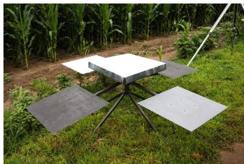
Figure 4.2 Ground truthing station for calibrating thermal imagery
