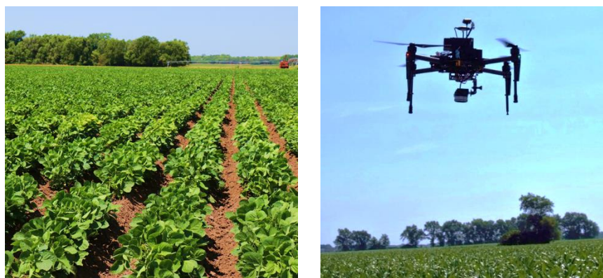
Figure 3.3. a) Soybean crop used for data collection. b) Matrice 100 with a Sony \alpha 5100 CIR camera
