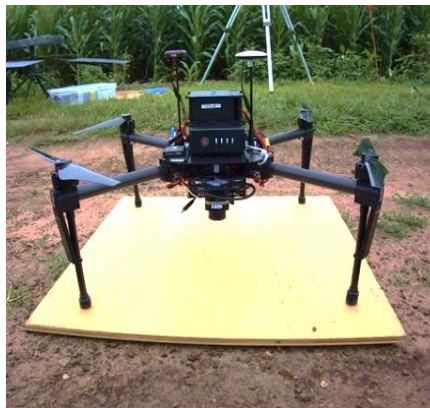
Figure 3.1. Matrice 100 quadcopter which was used for collecting infrared data
