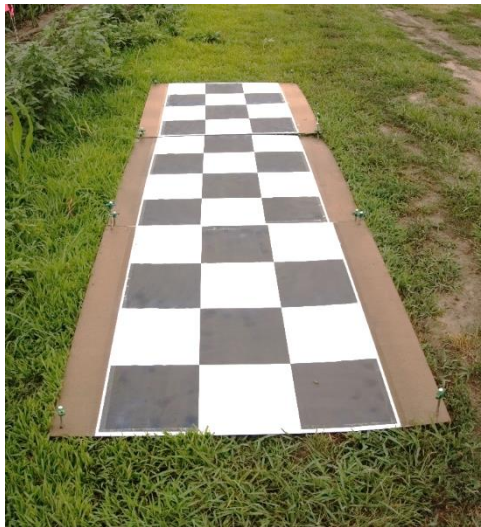
Figure 4.3 Checkerboard used for calculating RMSE for geometric accuracy
