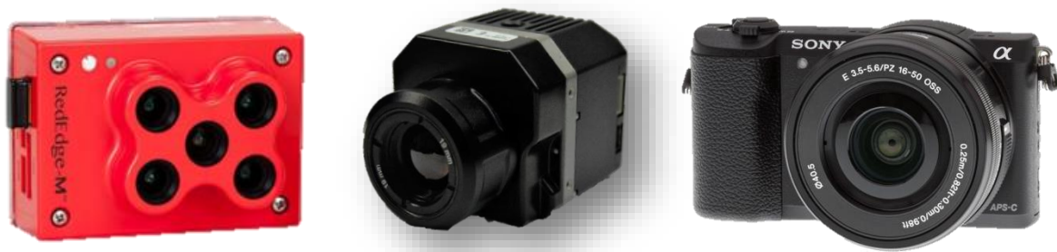
Figure 3.2. Camera sensor used for this study: a) Micasense Rededge-M b) Flir Vue pro R 13 mm c) Sony \alpha 5100 modified CIR
