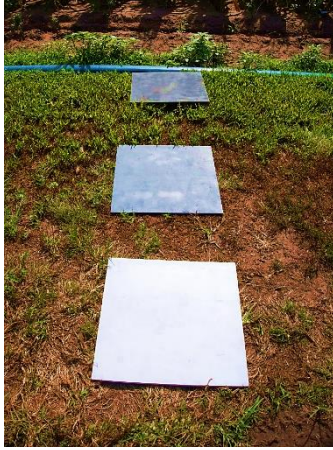
Figure 4.4 Wooden panels used to measure spectral discrimination
