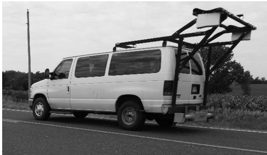
Figure 3-12 KDOT Laser crack measurement system
