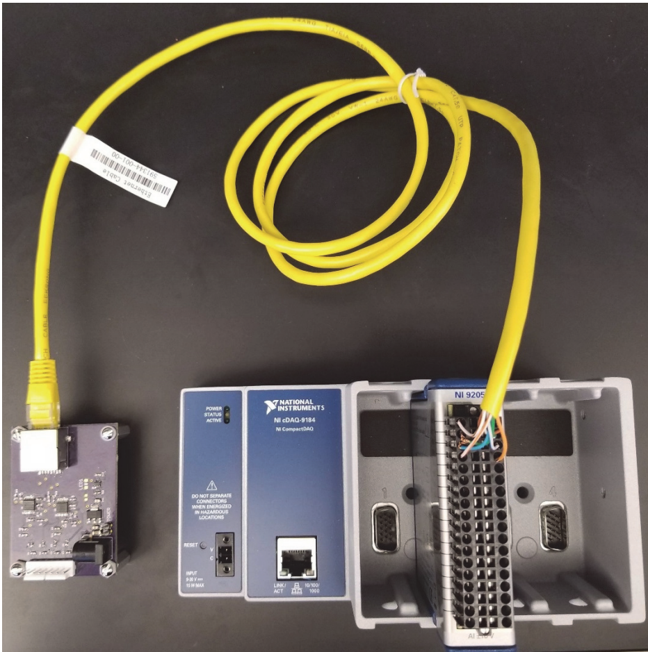
Figure 4-11. Connections between the version 2 analog conditioning circuitry, the NI 9205, and the NI 9184.
