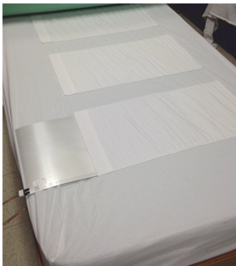
Figure 4-1. Example film sensor and pockets sewn into a fitted sheet that hold sensors in place. The mattress is turned upside down to illustrate EMFi sensor and pocket locations.
