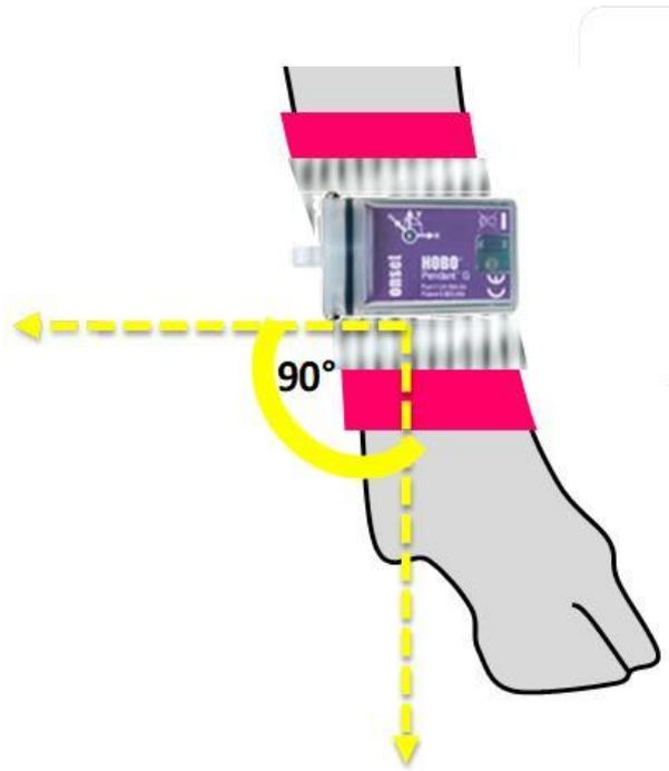
**Figure 2-6.** Rest logger is placed on calf's leg with purple side facing out. The y-axis of the logger lines up with the leg of the calf to insure proper orientation.
