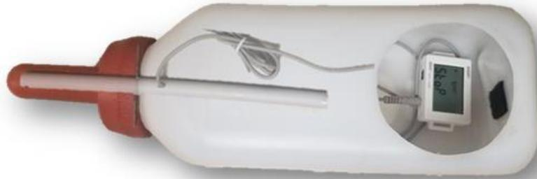
**Figure 2-1.** Environmental enrichment device (EED) contains a sensor (SW-18020P, ADAFruit, New York City, NY) housed within the bottle and dummy nipple. Calf use of the EED is automatically recorded on an event logger (UA-004-64; Onset Computer Corp., Bourne, MA) and data is downloaded periodically based on storage space, battery life, and study parameters.
