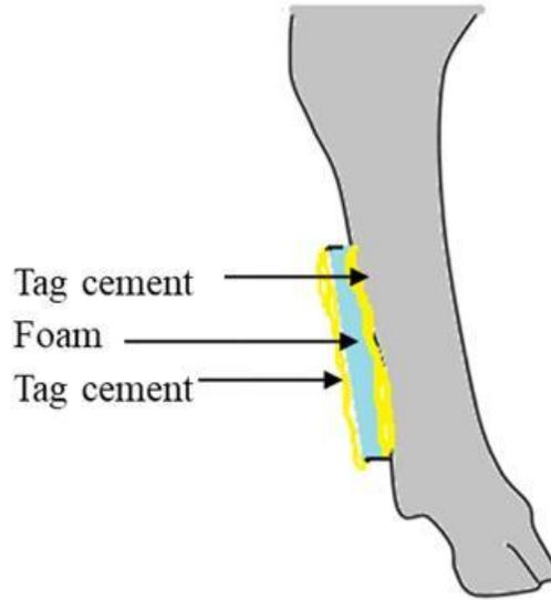
**Figure 2-2.** A 6.35 x 10.15 cm strip of foam non-slip drawer liner is attached to the calf's leg with a thin layer of tag cement. Liner is then wrapped with 2 layers of Vetwrap (3M Products, St. Paul, MN).
