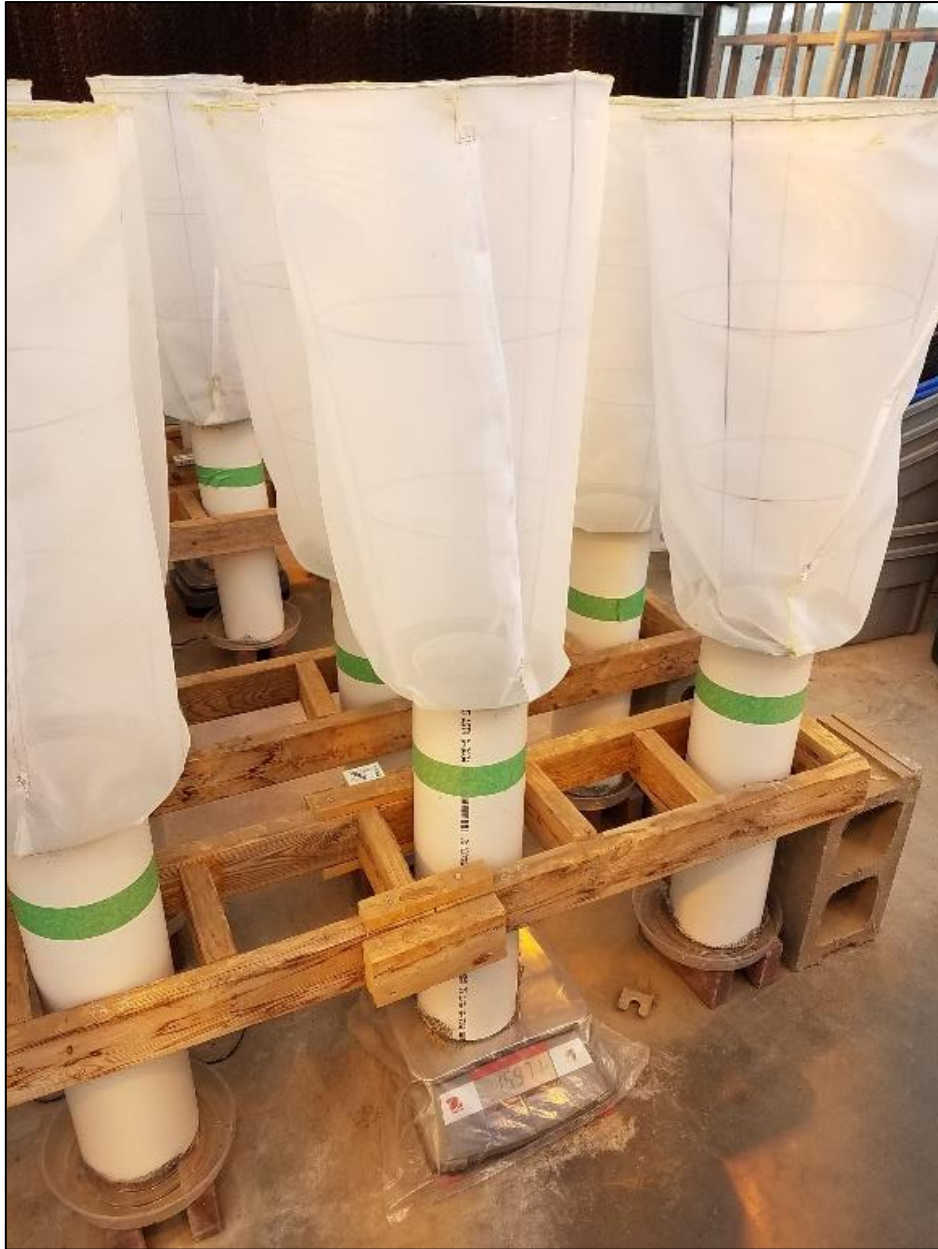
Figure 2.1 Cage, including exclusion enclosure and PVC soil column, sitting on top of an Ohaus® weighing scale.
