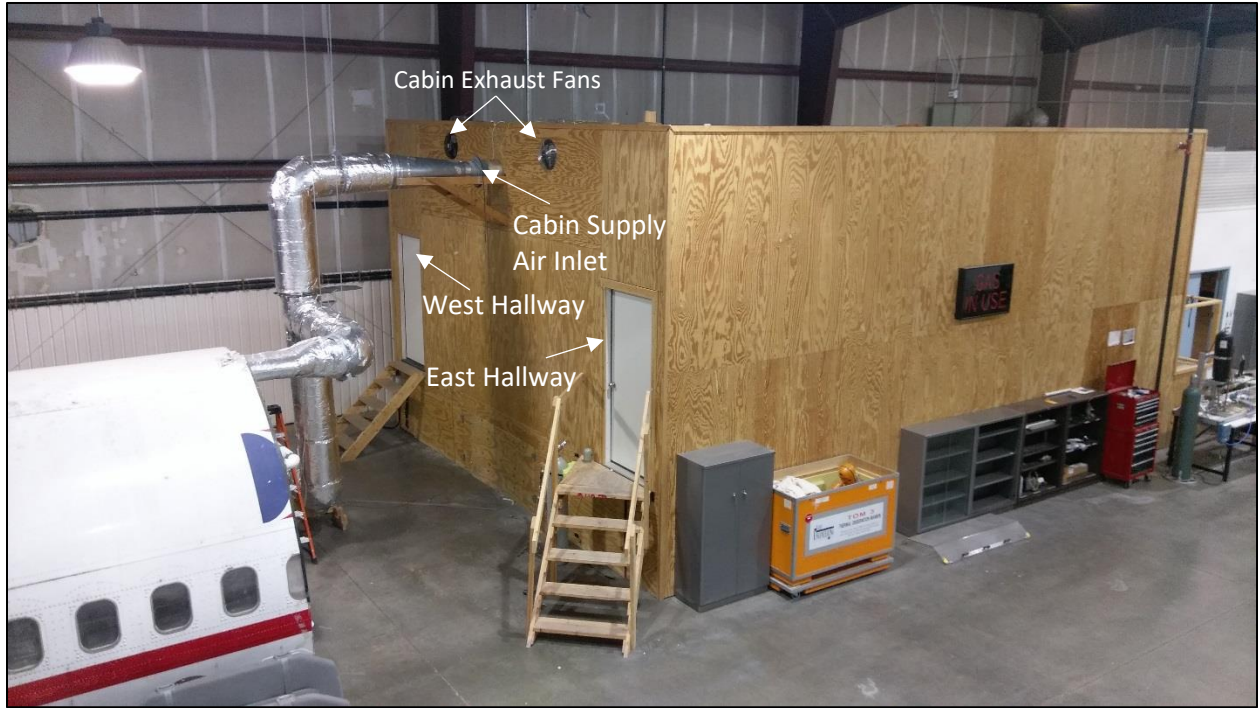
Figure 3.1 767 Mock-up Structure and Air Supply
