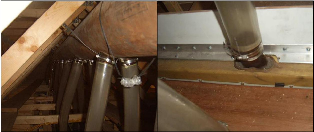
Figure 3.19 Boeing 767 Mock-up Supply Duct and Diffuser Connection (Patel, 2017)
