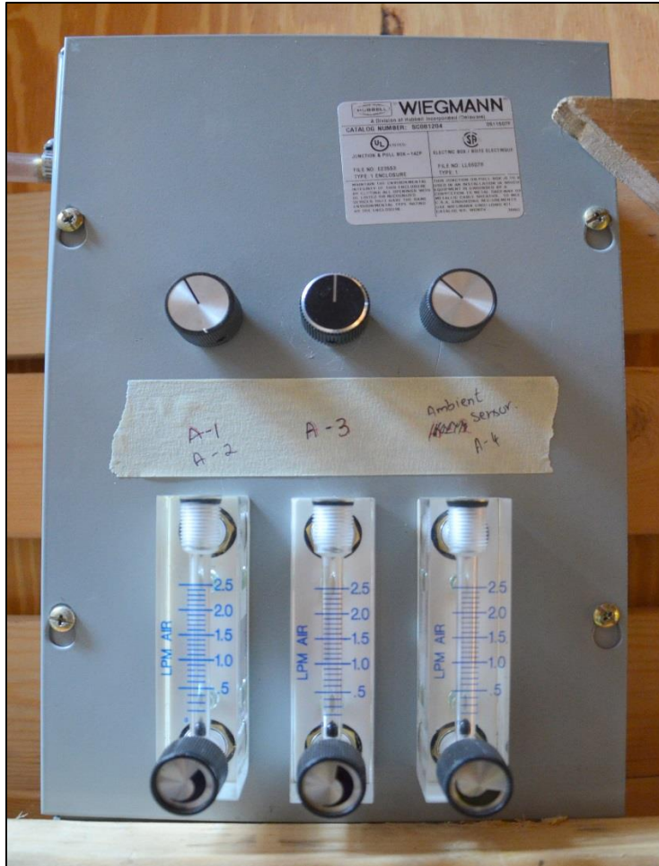
Figure 3.30 Flow Balancing System for CO 2 Analyzers (Patel, 2017)
