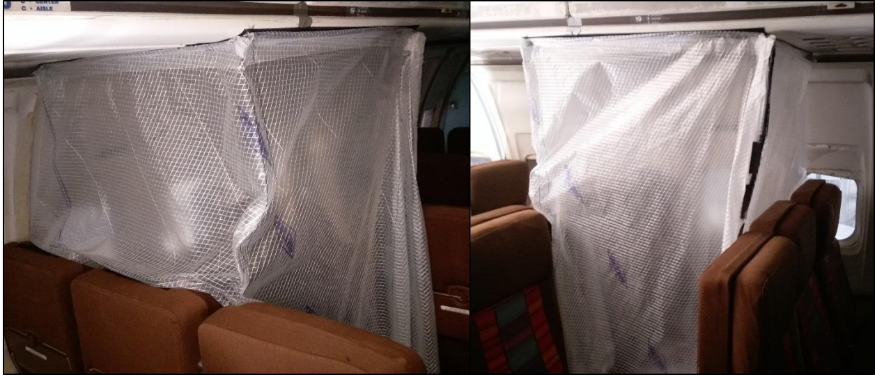
Figure 4.1 ISOPASS Installed in Cabin
