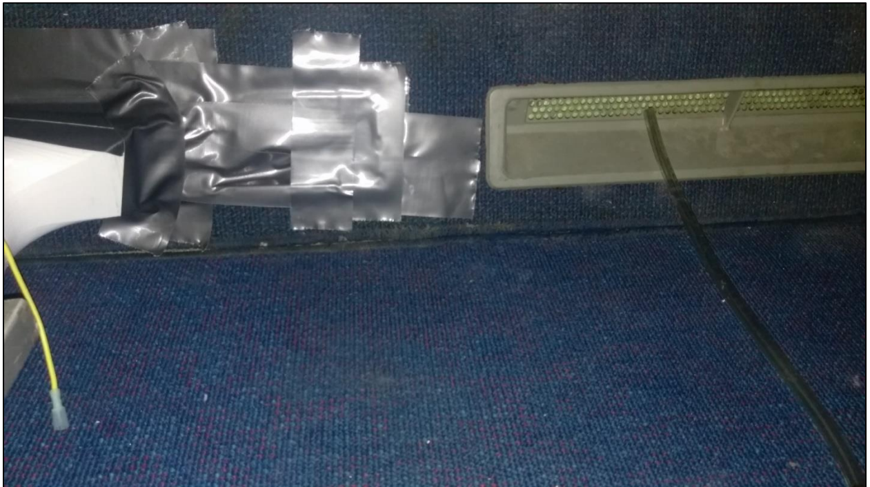
Figure 4.41 Vent After ISOPASS Exhaust Exit, 737 Cabin
