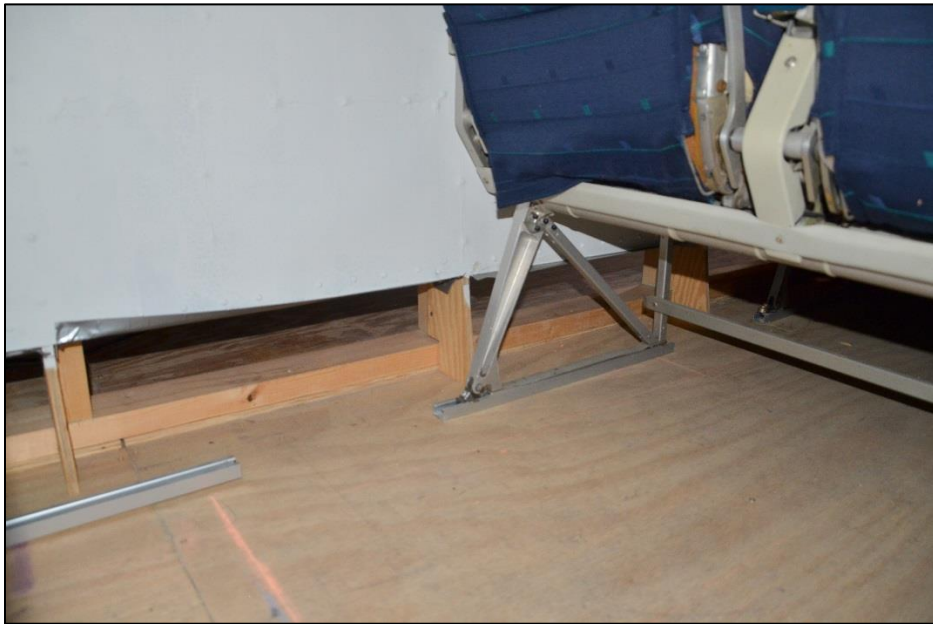
Figure 3.5 Ventilation Gaps Inside 767 Mock-up (Patel, 2017)
