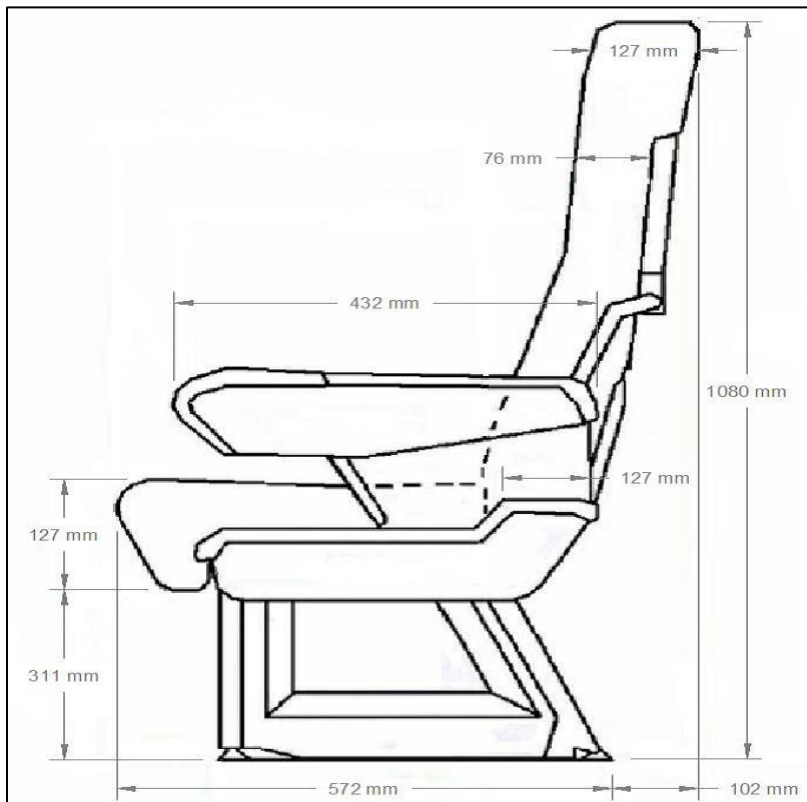
Figure 3.9 Boeing 767 Seats Side View Dimensions (Trupka, 2011)
