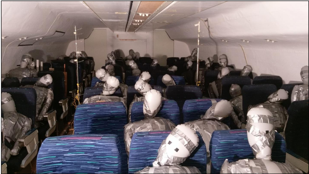
Figure 3.17 Boeing 767 Mock-up with Mannequins
