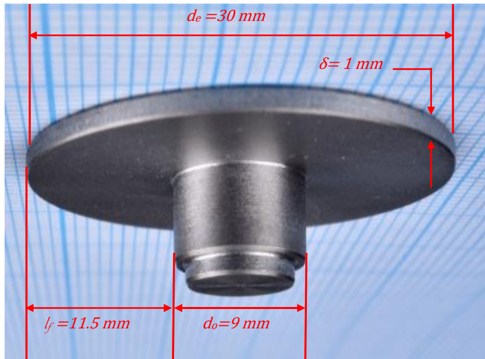
Figure 5.6: The design of the fin used in this work.
