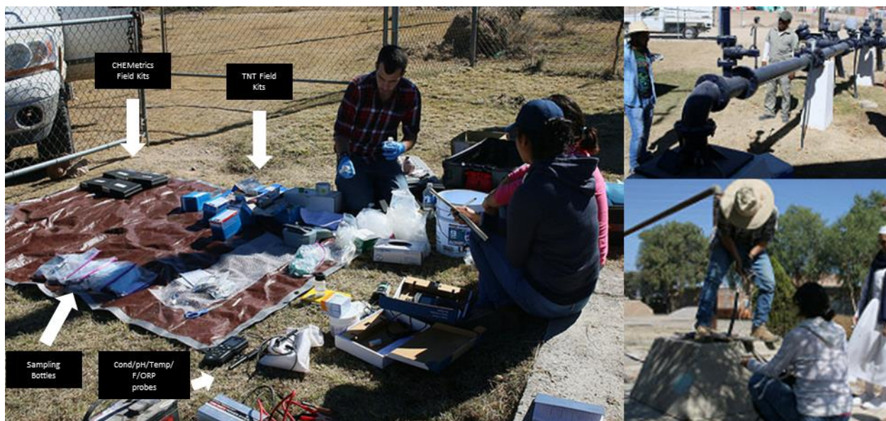
Figure 3.1 Images of production wells sampled, the preparation of field kits for conducting analysis, and collecting depth to water measurements in the IBAS in Mexico (Images courtesy of William Thurston at Caminos del Agua).
