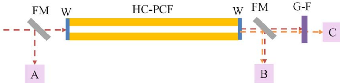
Figure 4.29: Simplified version of the setup of pump coupling into HC-PCF and measuring pump pulse energy as well as residual pump and mid-IR laser pulse energies.
