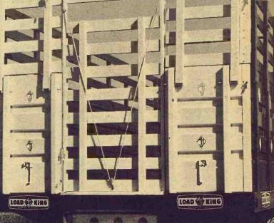
The Load King specially designed understructure has built-in clearance frame for hoist, eliminating the need to cut across members. The platform has a heavy duty reinforced framed opening for convenient hoist mounting. Flooring fastened from underneath; no bolt heads to protrude, no depressions to cause splintering and rotting. Get the truck bed that's built by Kansans, distributed by Kansans — Used by Everyone.
