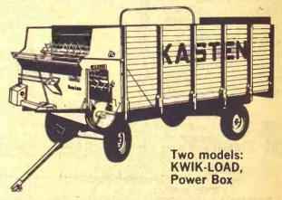
Brand new shipment of Kasten forage boxes -- the most for your money considering design and ruggedness. Sweep speed on KWIK-LOAD model saves 3 minutes at each unloading, permits an extra load per day. Both models use deep, 16-inch-auger cross conveyor with 6-inch flights for speedy unloading from the left side.
