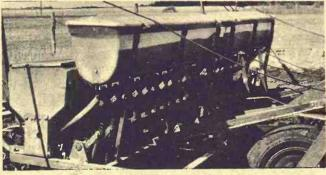
Multi-use dispenser fits most tillage equipment. Mighty handy when you want to spread fertilizer, insecticides, weed killers, root worm controls, or when auguring or seeding. In fact, ideal for even dispersing of any granular or pellet, soil or crop treatment. Built to last. Highly corrosive-resistant fiberglass box with aluminum or synthetics in other parts. Easily adjustable, controlled application. Trouble free operation. Three box lengths available.
