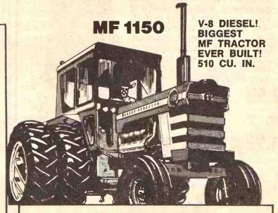
First big row-crop tractor with a V-8 diesel. Power and speed to spare. Moves big implements 5 to 7 mph. 12-speed Multi-Power transmission, hydrostatic power steering, tilt/telescope steering wheel standard. Handles like a small tractor. Worth a fleet of ordinary tractors!
