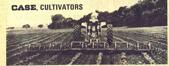
Model B trail-type rotary hoe for 6 rows, is also available in 2, 3 and 4-row sizes. Row sections are 42 inches wide.
