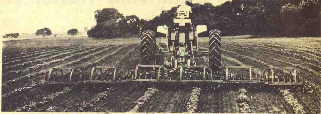
Model B trail-type rotary hoe for 6 rows, is also available in 2, 3 and 4-row sizes. Row sections are 42 inches wide.
