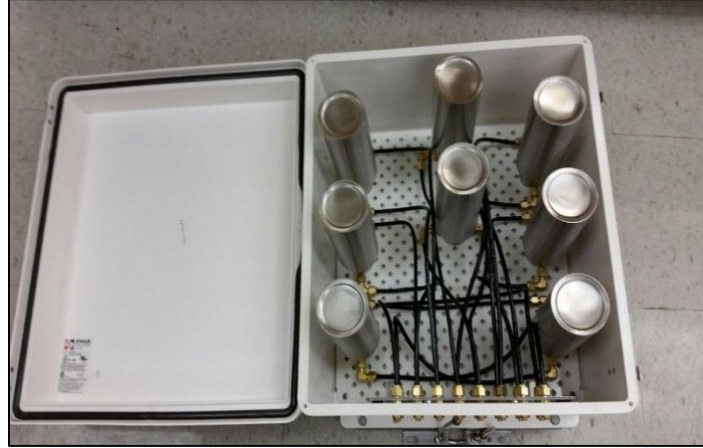
Figure 2.1 – A picture of the buffering volumes (metallic flasks) used with the multi-port sampling system.
