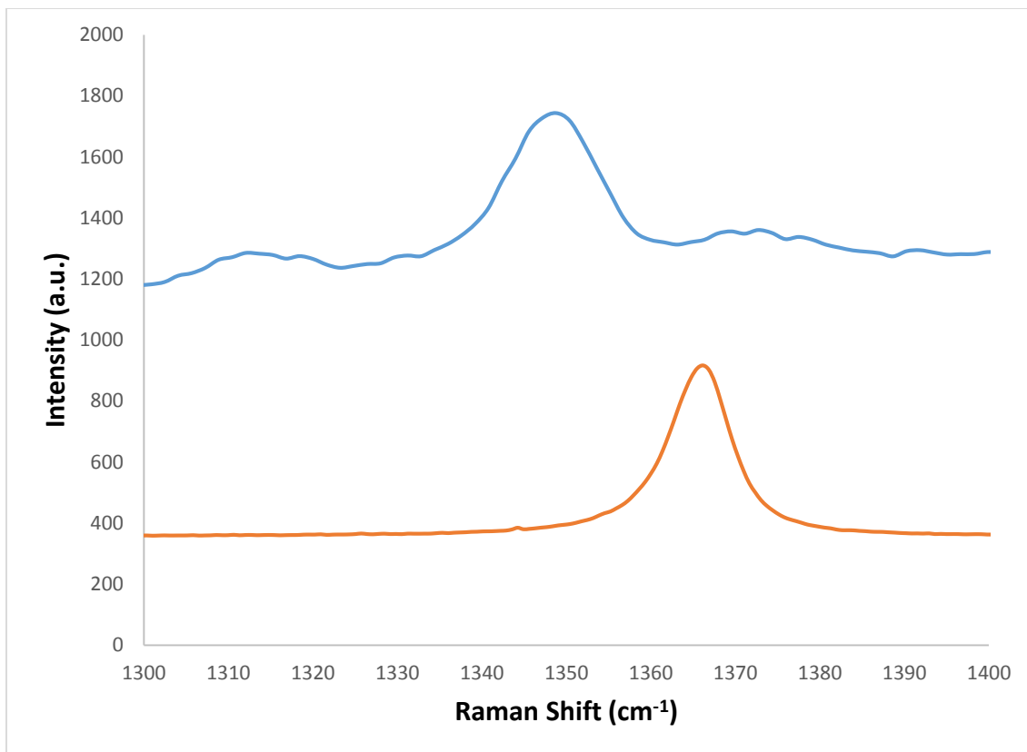
Figure 4-17 Raman shift of exfoliated hBN powder (blue) from bulk hBN Raman signature (orange).
