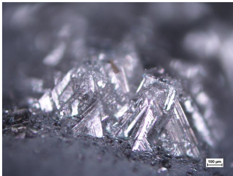
Figure 4-1 Sample 1 from stepped temperature growth experiments. Crystals grown vertically, merging into each other to create pyramid like morphologies.
