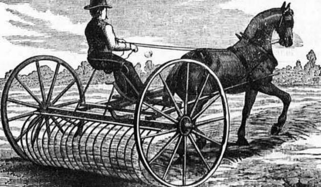
Patented Aug. 1867, Jan. 1876, June 1876, and Nov. 1876. 80,000 now in Use. Twenty Steel Teeth. No complicated ratchet wheels, friction bands, nor other horse machinery needed to operate it. Right touch of lever and DRIVER'S WHEEL dumps it. Best self dump in market. A small boy rakes easily 20 acres per day with the COATES' "LOCK LEVER." Send for Circulars. A. W. COATES & CO., ALLIANCE, OHIO.
