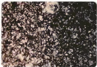
Figure 1. Photomicrograph of Brownville Limestone Member (Sample Sl-A, X10, crossed nicols). Note low diversity of taxa and abundance of quartz grains.
