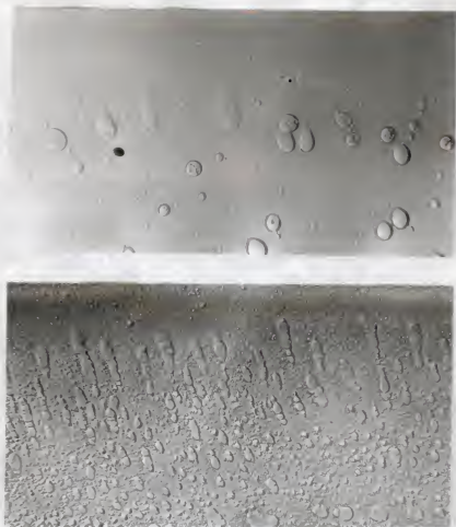
Fig. 10. The action of water on the complex coacervate of starch-chloral hydrate gelatin which is produced by the action of NaCl solution. Upper, excessive amounts of water rapidly destroyed the coacervate droplets; lower, the coacervate droplets were reproduced by fan-drying for 15 minutes. Mag. 198X
