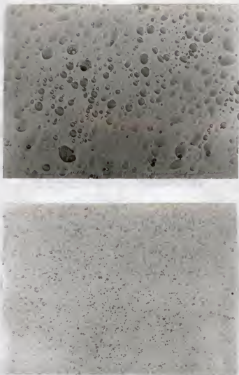
Fig. 6. Upper, coacervate droplets formed by mixing 4% amylo maize in 6 M chloral hydrate and 4% gelatin solution (1:1); lower, coacervate droplets of amylopectin-gelatin by same procedure as described above. Mag. 136X.
