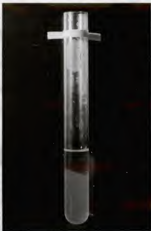
Fig. 4. Coacervate (Bottom Layer) formed by mixing 4% starch in 6 M chloral hydrate with equal amount of 4% gelatin solution at pH 3.5.
