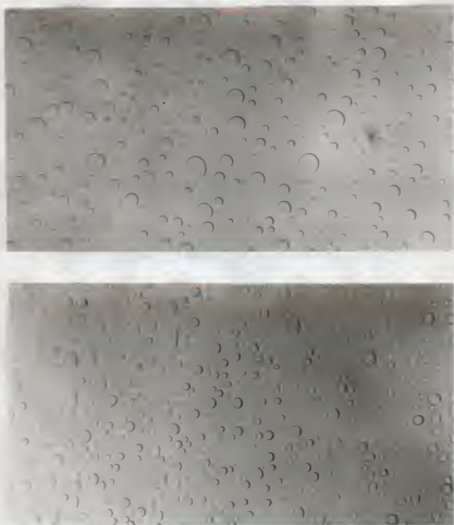
Fig. 9. Complex coacervate of starch-chloral hydrate gelatin formed by the action of \text{Na}_2\text{SO}_4 (upper) or \text{Na}_3\text{PO}_4 (lower). One drop of 0.01% \text{Na}_2\text{SO}_4 or \text{Na}_3\text{PO}_4 solution was added to the mixture of 4% starch in 6 M chloral hydrate and 4% gelatin. Mag. 198X
