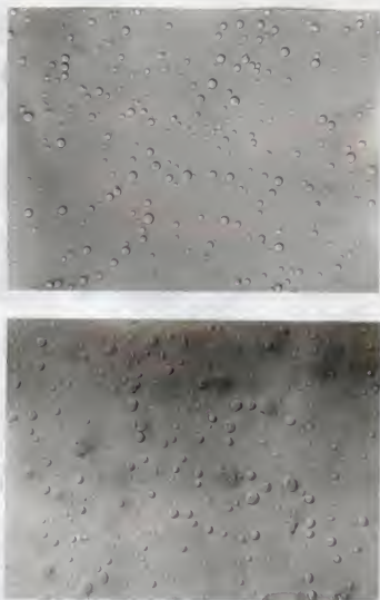
Fig. 5. Upper, coacervate droplets obtained after dilution of 4% starch in chloral hydrate and 4% gelatin (1:1) at pH 3.5 with an equal amount of water; lower, same as upper but coacervate was warmed to 40°C for one minute. KI-I 2 stained. Mag. 198X
