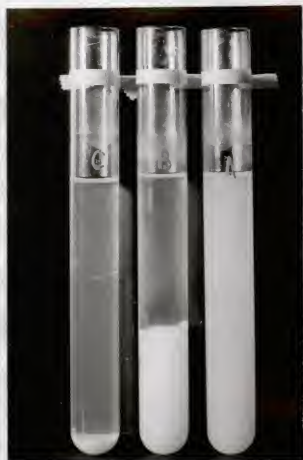
Fig. 1. Precipitate of amylose-chloral hydrate complex formed after dilution of a 4% amyloamize (A), 4% defatted starch (B) or 4% amylopectin (C) in 6M chloral hydrate with 10 parts of distilled water.
