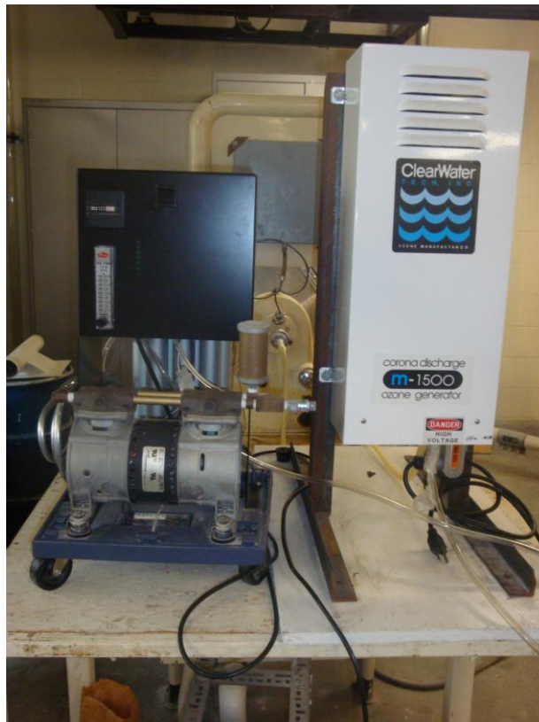
Figure 1. Pilot scale ozone generator and oxygen generator
