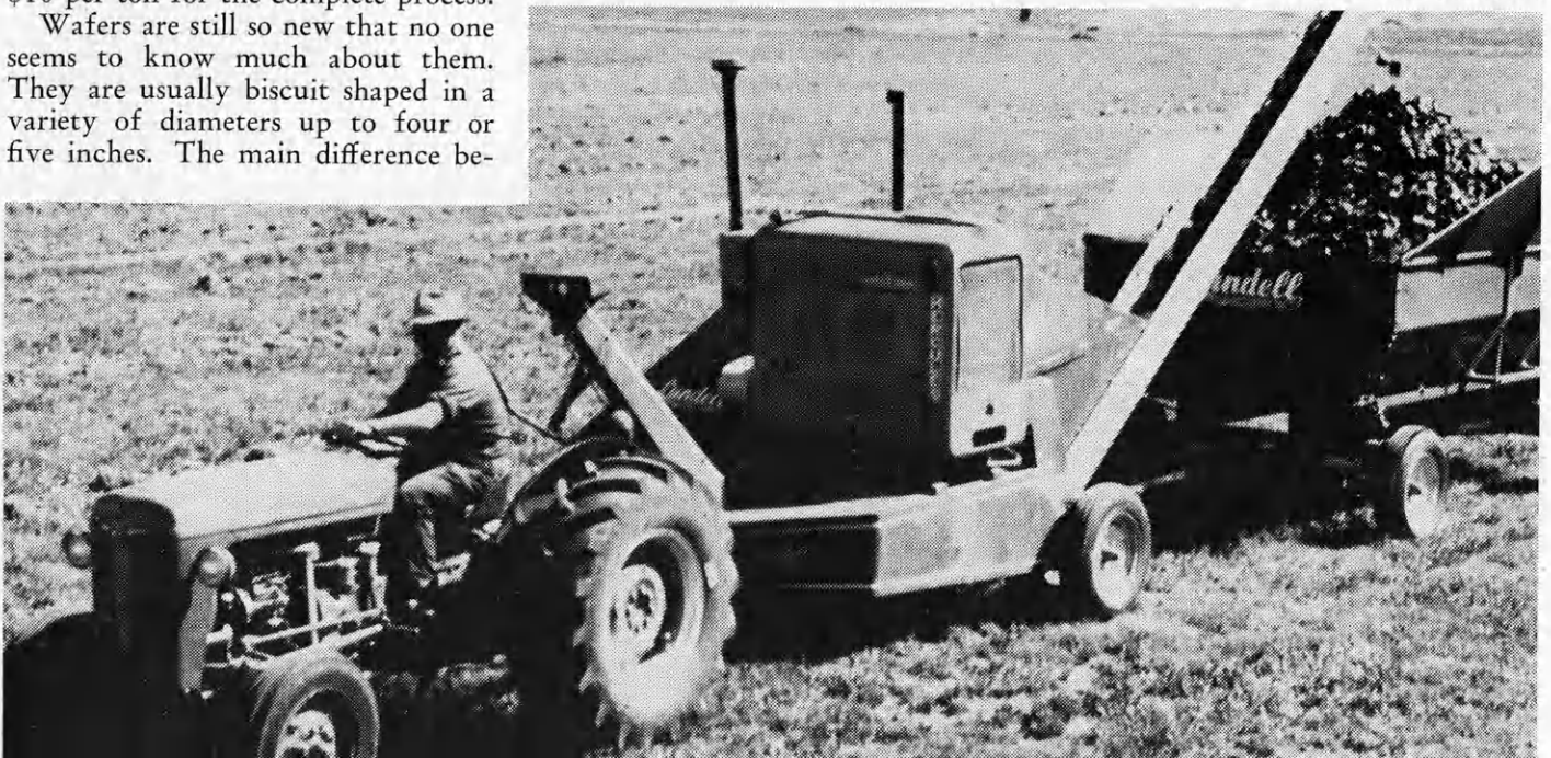
Wafer machines like this are becoming popular. The hay is compressed into round or cube shapes which can be handled with grain elevators. This saves you time and labor.
