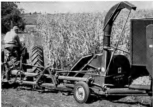
Here's the leading flywheel-type field harvester—the big McCormick No. 36! It chops over 45 tons of corn silage per hour. Pto or engine drive.
