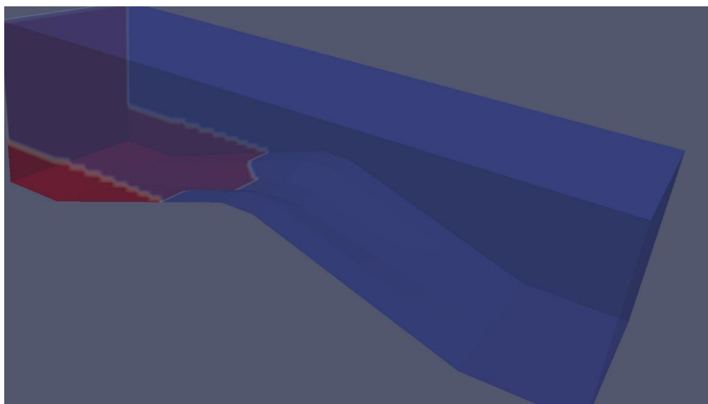
Figure 37. Initial conditions for the smooth dam with auxiliary spillway
