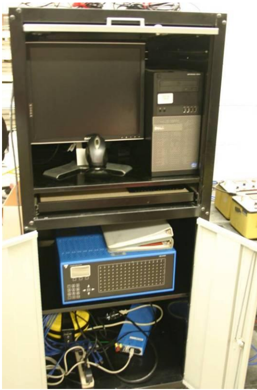
Figure 3.7 Data acquisition system for recording measurements
