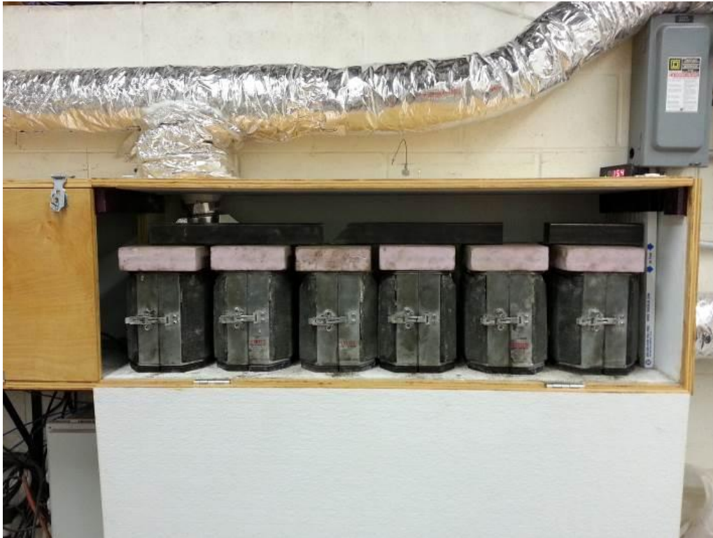
Figure 5.11 Air-conditioned box used to match-cure
