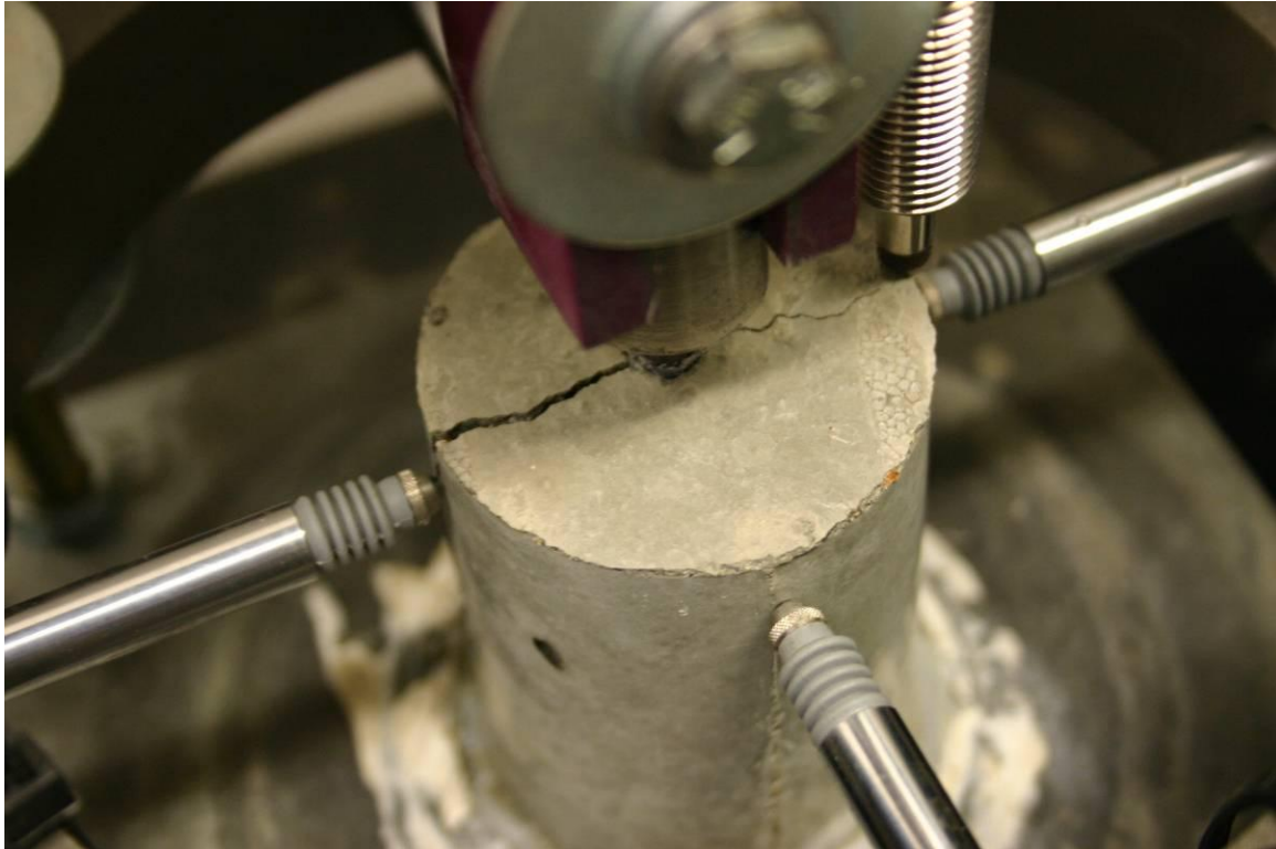
Figure 11.6 WH specimen after testing with cracking
