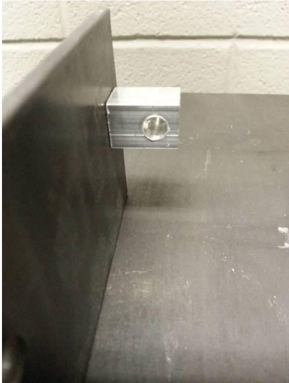
Figure 11.16 Aluminum insert to secure VWSG in position
