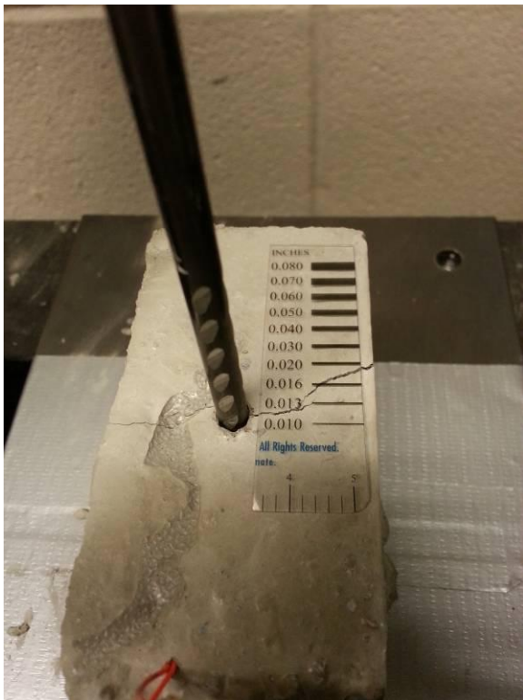
Figure 12.4 Shallow 15-degree indent specimen after testing
