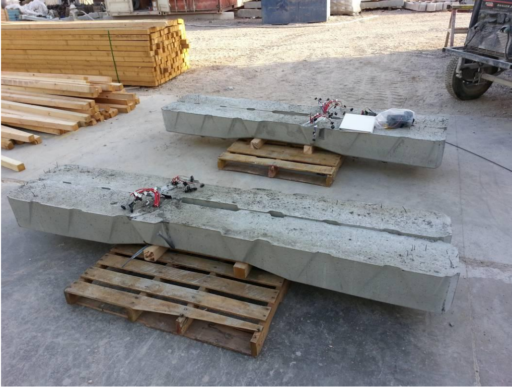
Figure 14.14 Crossties after being cut and loaded onto pallets
