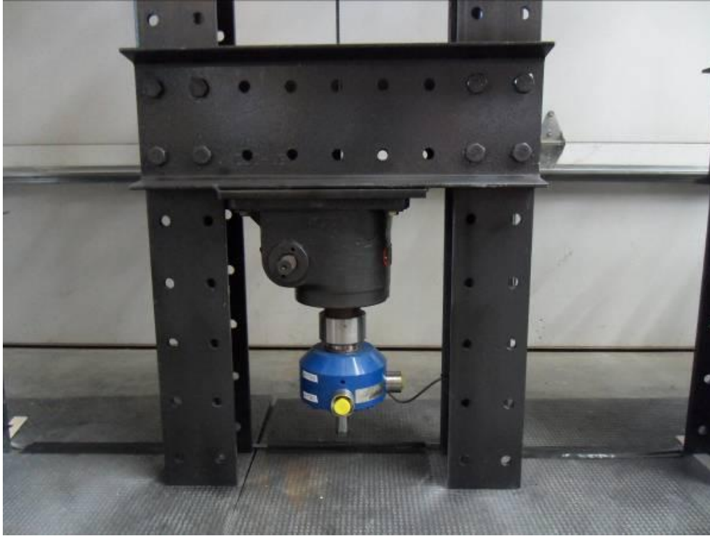
Figure 3.4 Plate load cell attached to bottom screw jack
