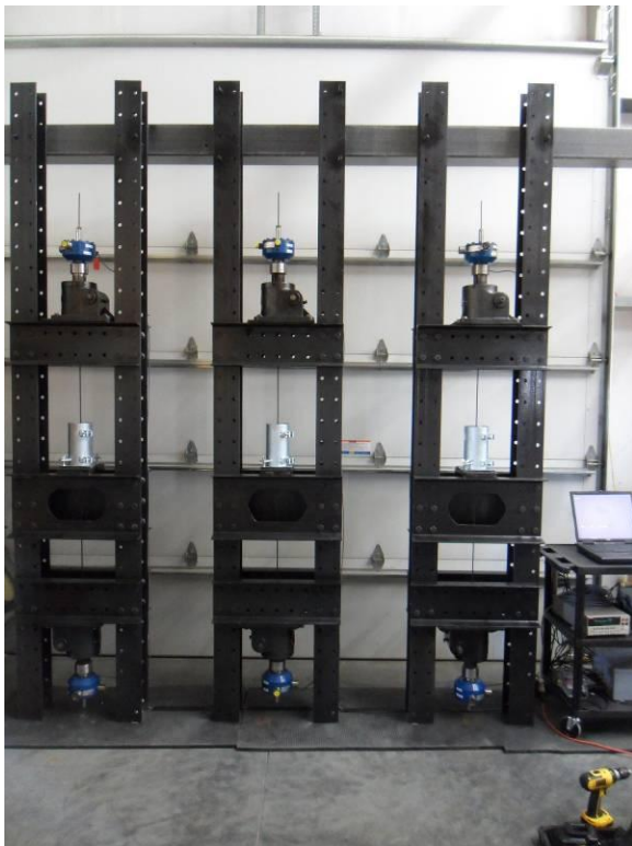
Figure 3.2 Frame setup involving screw jacks on top and bottom of frames
