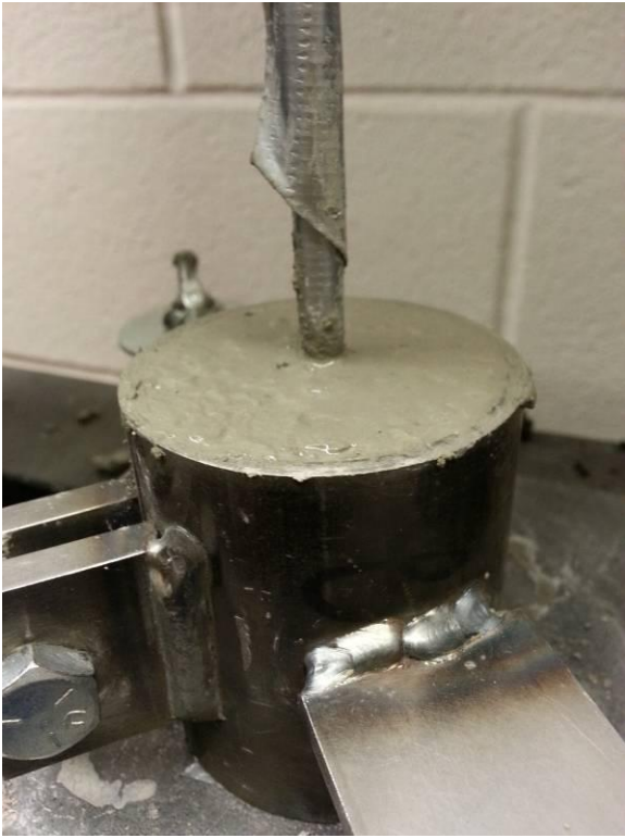
Figure 9.4 2-inch-diameter specimen after being cast
