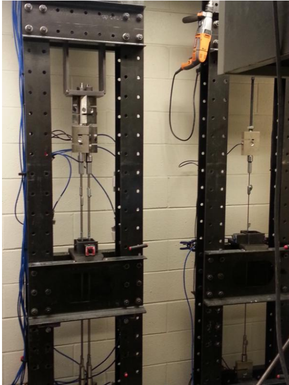
Figure 13.1 4-wire and single wire frame setup
