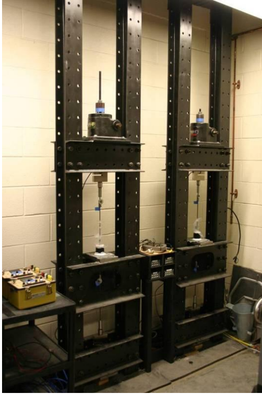
Figure 3.1 Frame setup involving a screw jack at the top of the frame
