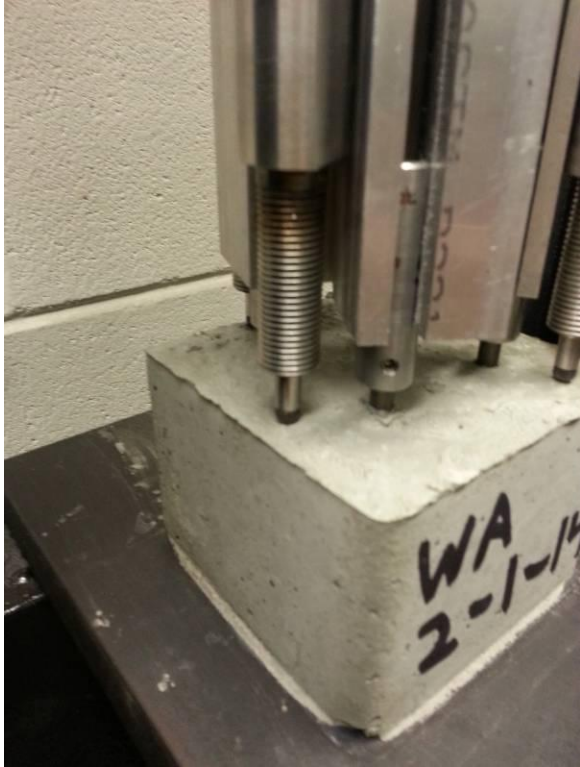
Figure 13.7 WA 4-wire specimen after testing
