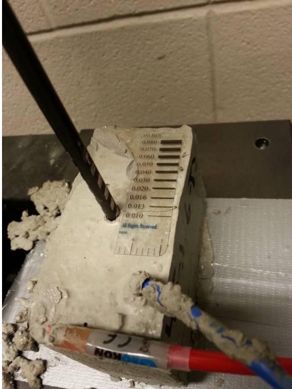
Figure 12.16 Deep 45-degree indent specimen after testing
