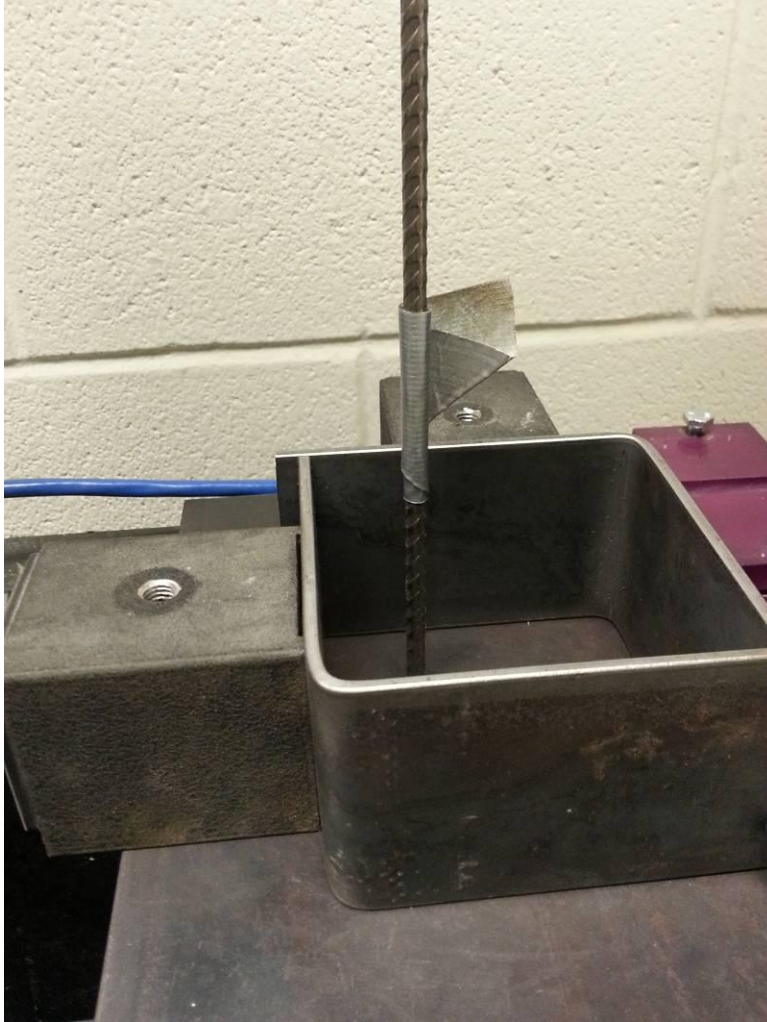
Figure 13.3 Single wire specimen before casting
