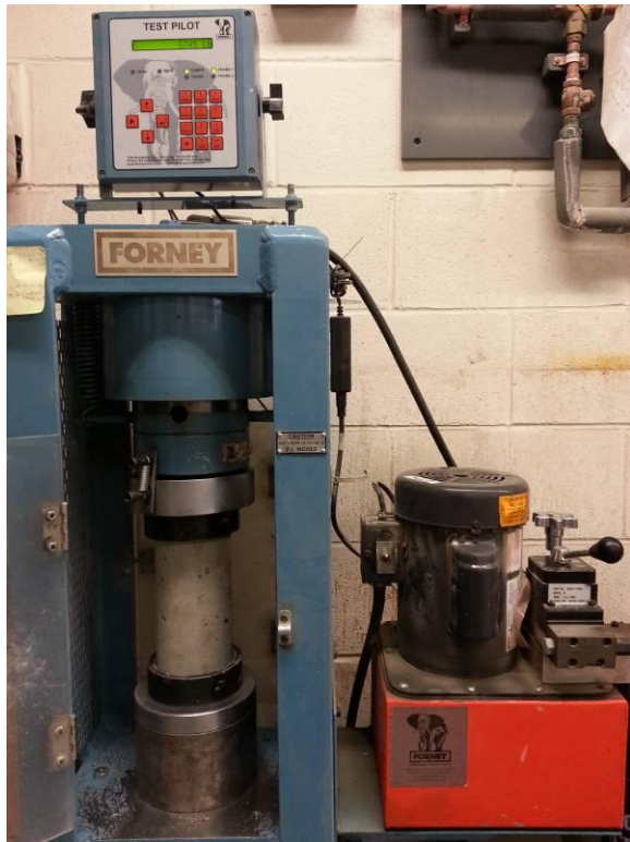
Figure 5.13 Compression cylinder being tested
