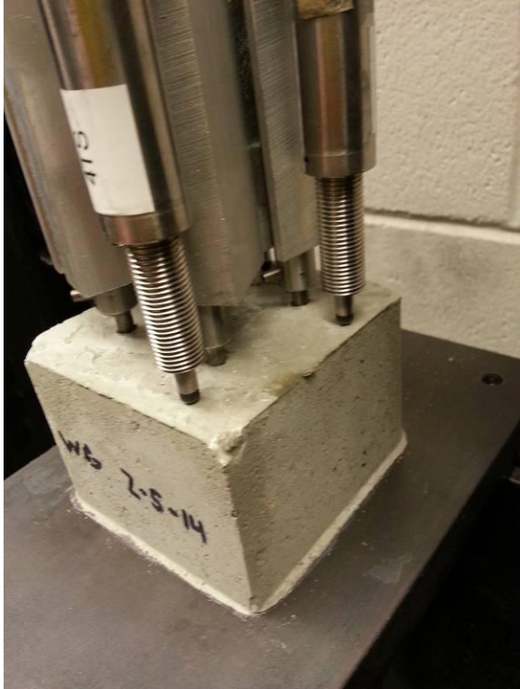
Figure 13.13 WG 4-wire specimen after testing
