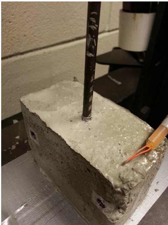
Figure 12.14 Shallow 45-degree indent specimen after testing
