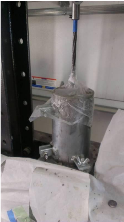
Figure 5.8 Finished test specimen covered with plastic
