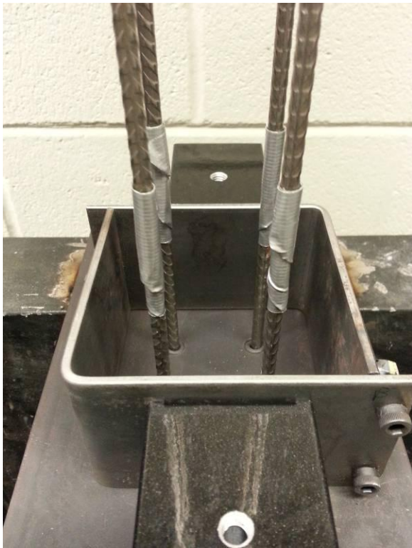
Figure 13.2 4-wire specimen before casting
