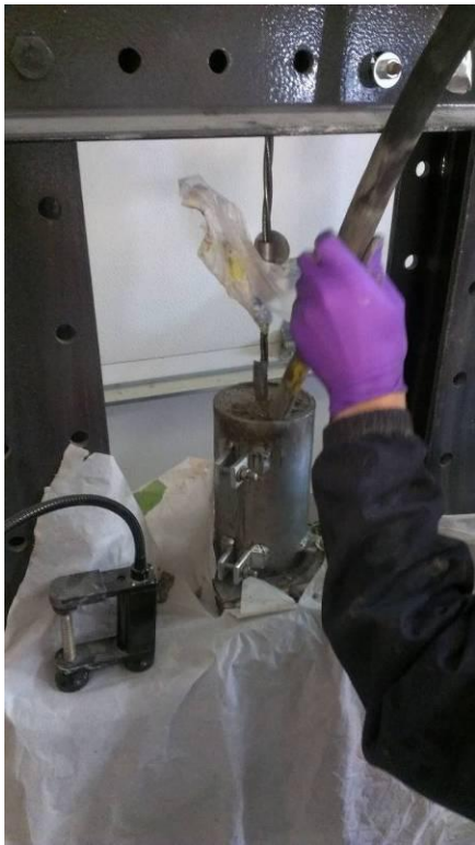
Figure 5.6 Test specimen being vibrated
