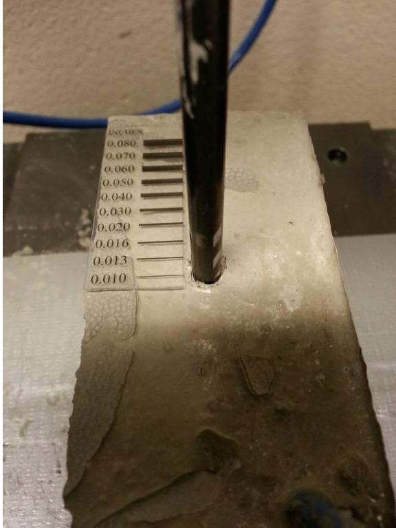
Figure 12.9 Shallow 30-degree indent specimen after testing
