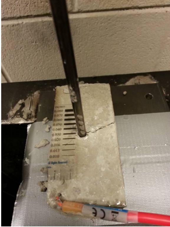
Figure 12.6 Deep 15-degree indent specimen after testing
