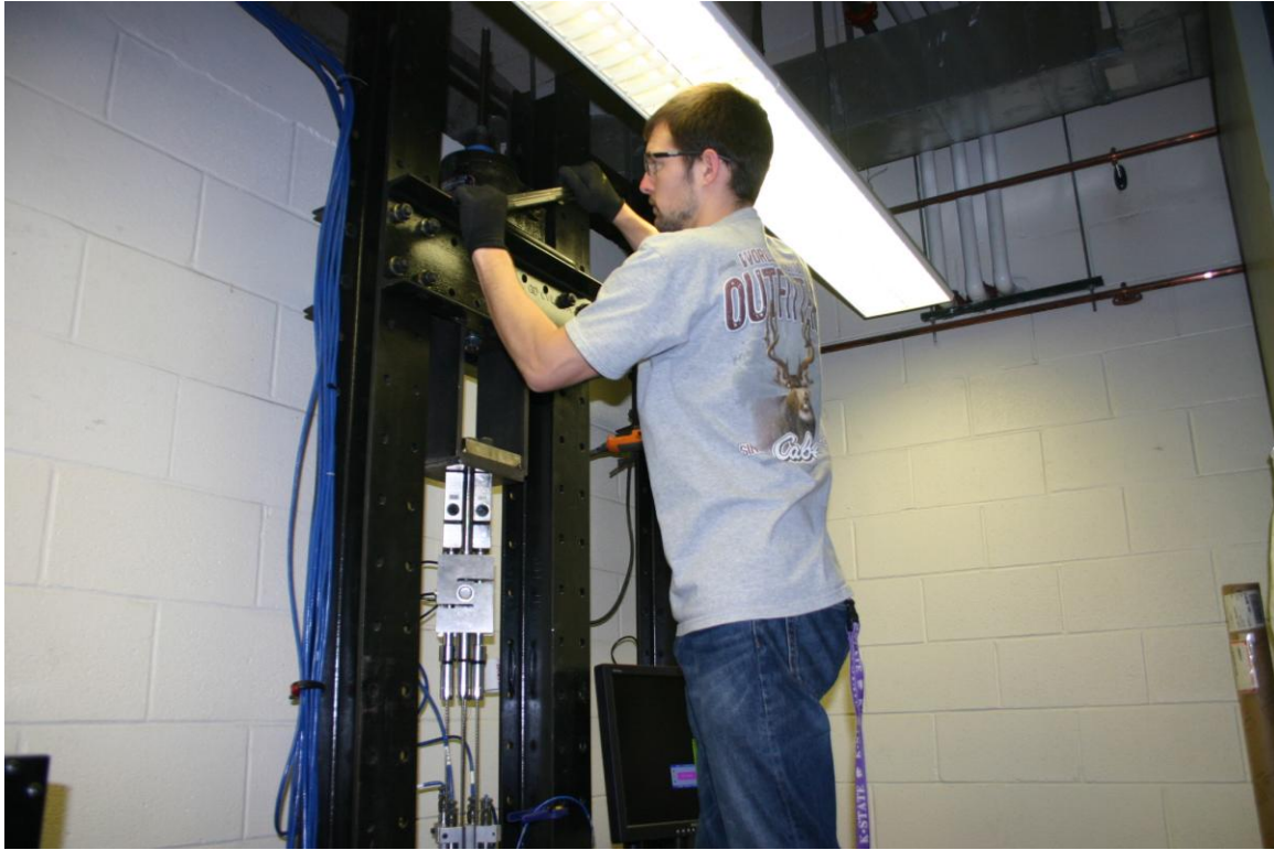
Figure 7.5 Top jack shaft being turned during testing
