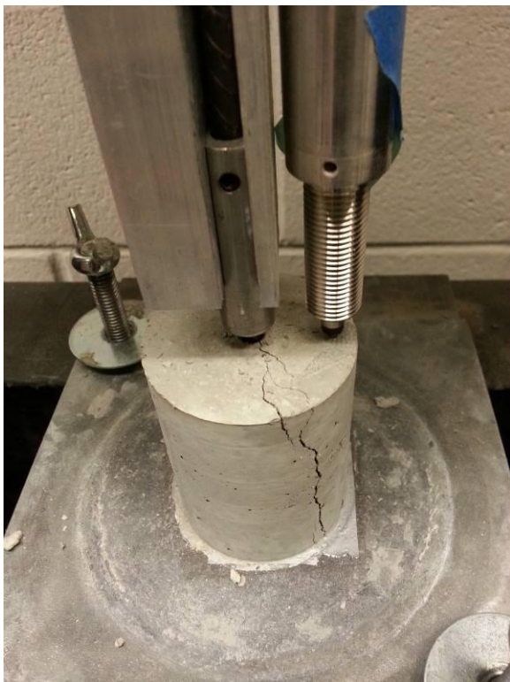
Figure 9.15 Cracked 2-inch-diameter unconfined specimen after testing
