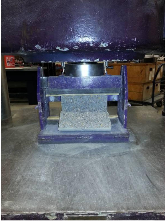
Figure 5.14 Split tensile specimen after testing
