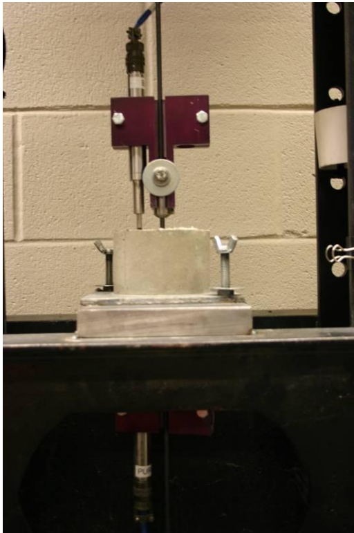
Figure 3.6 LVDT setup to measure end-slip
