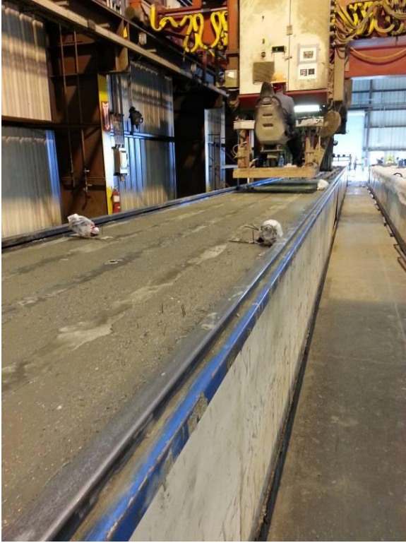
Figure 14.10 Crosstie after being cast
