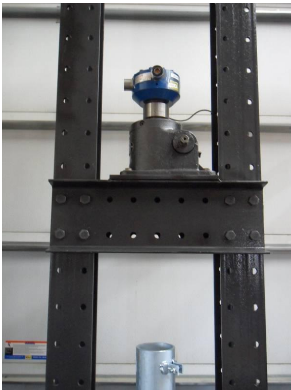
Figure 3.5 Plate load cell attached to top screw jack
