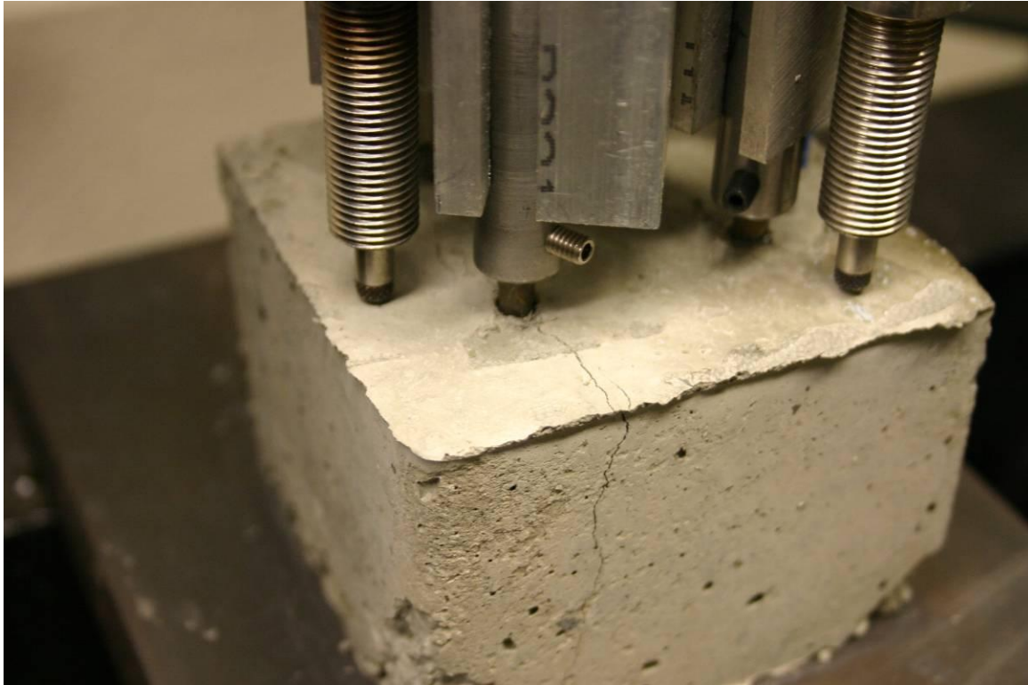
Figure 13.32 Cracking of specimen with glass fiber mesh located off the wire
