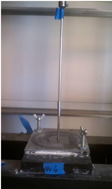
Figure 7.1 Bond break and straw on wire
