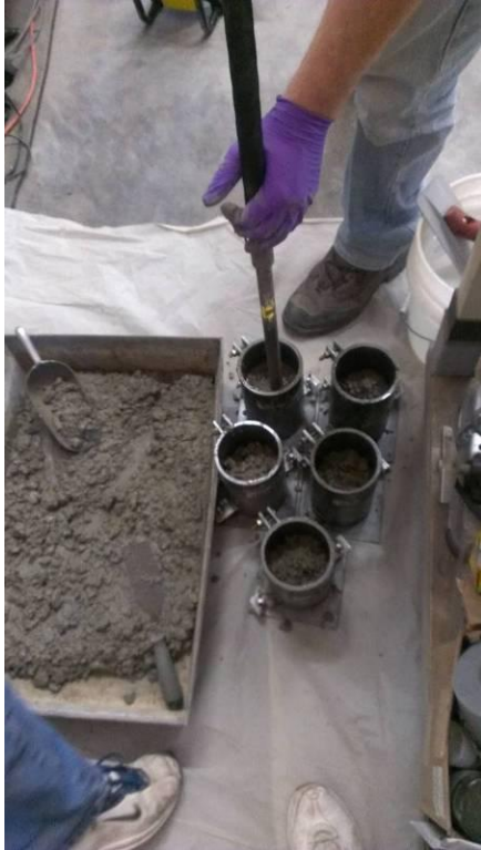
Figure 5.5 Strength cylinders being vibrated
