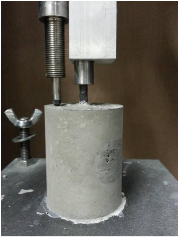
Figure 9.9 2-inch-diameter unconfined specimen before testing
