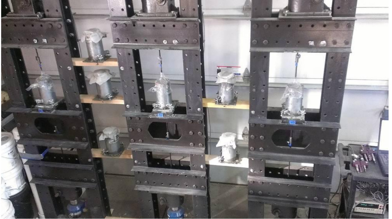
Figure 5.10 Strength cylinders curing next to test specimens
