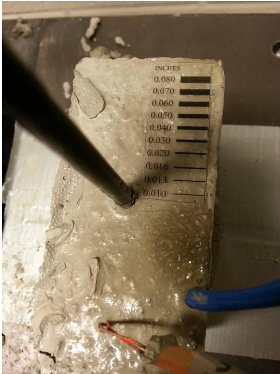
Figure 12.29 Shallow 90-degree indent specimen after testing
