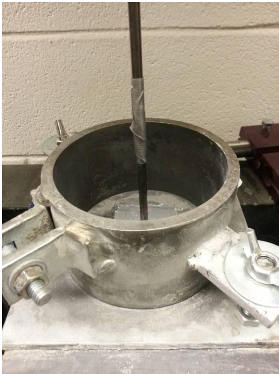
Figure 9.2 4-inch-diameter specimen mold
