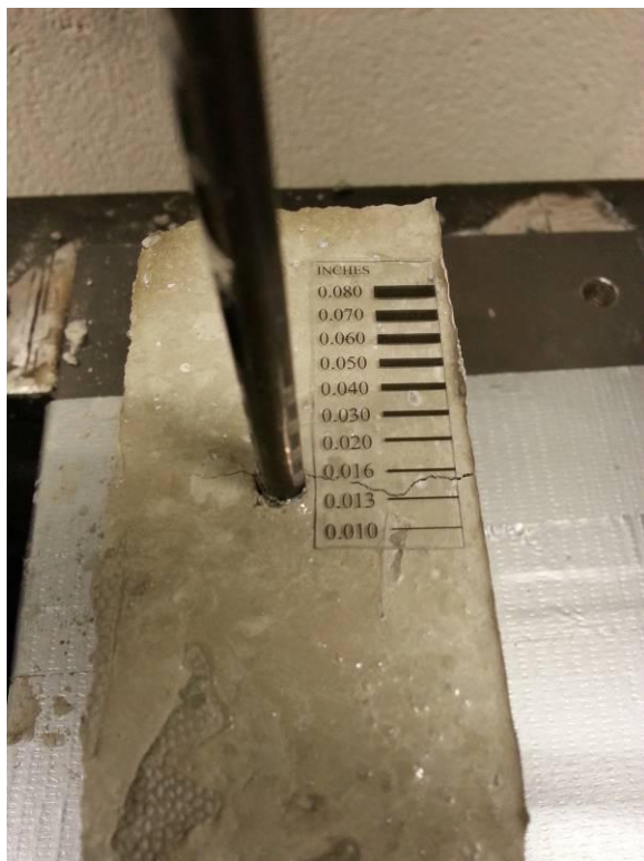
Figure 12.31 Deep 90-degree indent specimen after testing
