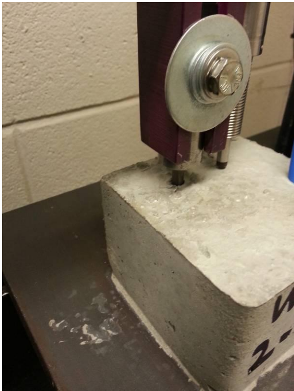
Figure 13.8 WA single wire specimen after testing
