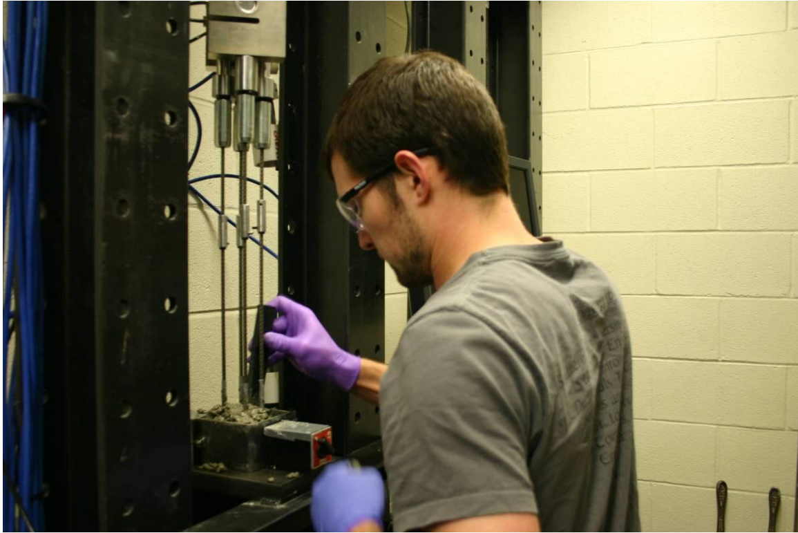
Figure 5.9 Smaller test specimen being rodded
