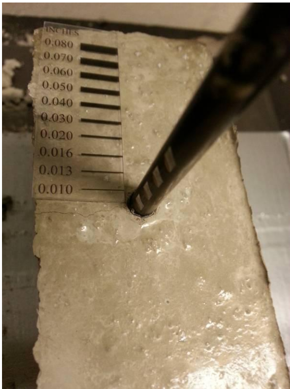
Figure 12.21 Deep 60-degree indent specimen after testing
