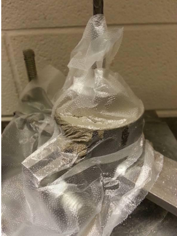
Figure 9.5 2-inch-diameter specimen covered with plastic after casting
