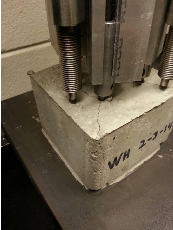
Figure 13.15 WH 4-wire specimen after testing
