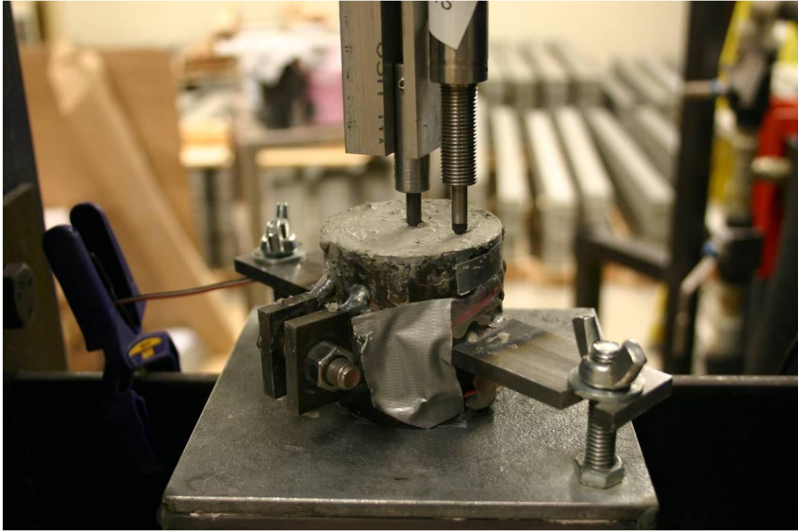
Figure 9.8 2-inch-diameter confined specimen before testing
