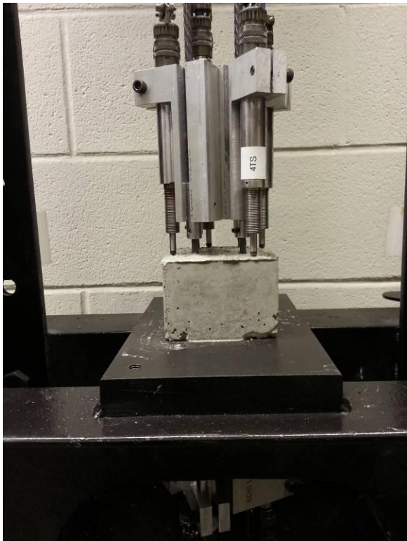
Figure 13.5 Top LVDT locations for 4-wire specimen test
