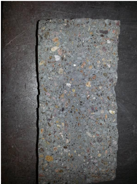
Figure 5.15 Close-up of split tensile specimen after failure
