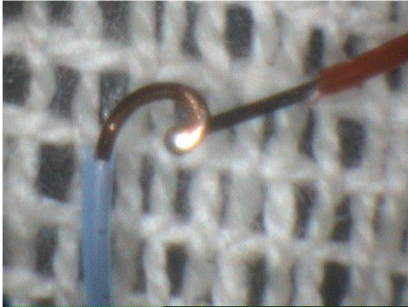
Figure 4.4: Un-insulated Thermocouple Stitched on Woven Fabric
