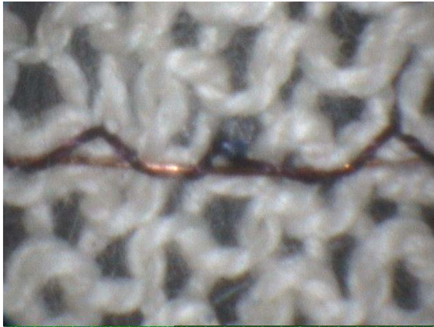
Figure 4.12: RTD Stitched on Knitted Fabric
