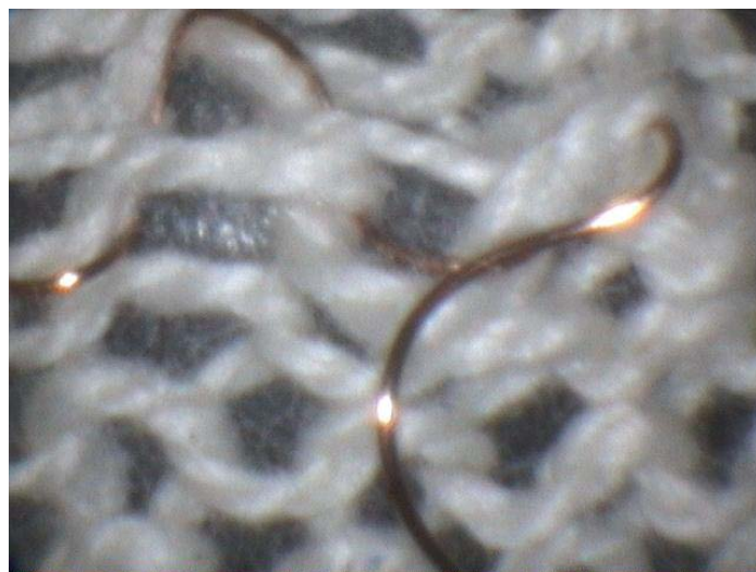
Figure 4.11: RTD Sensor Interlaced into Knitted Fabric
