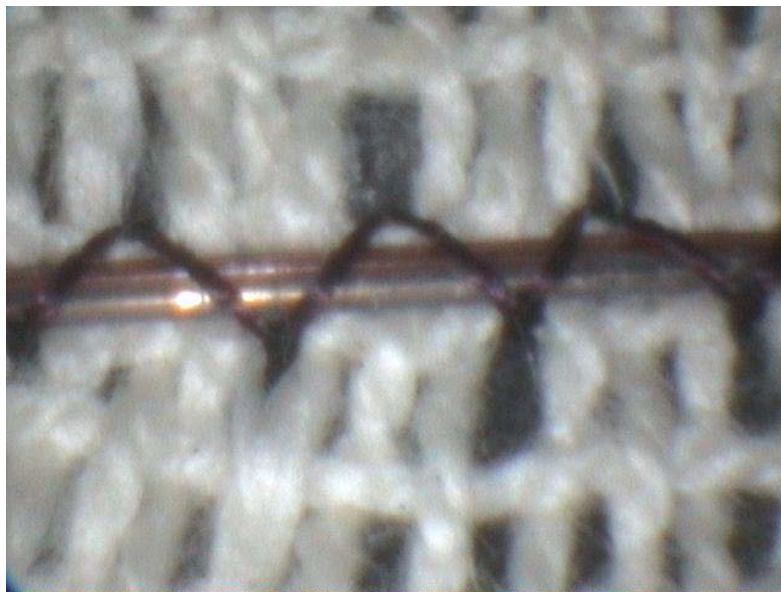
Figure 4.2: Insulated Thermocouple Stitched on Woven Fabric
