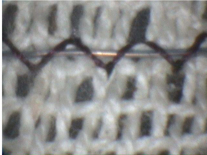
Figure 4.10: Un-insulated Thermocouple Stitched on Knitted Fabric
