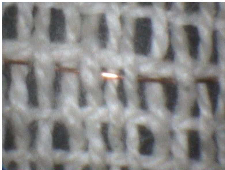
Figure 4.5: Woven in RTD in Woven Fabric
