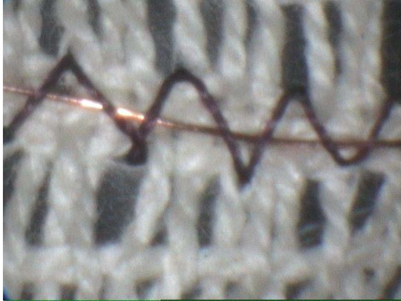
Figure 4.6: RTD Stitched on Woven Fabric
