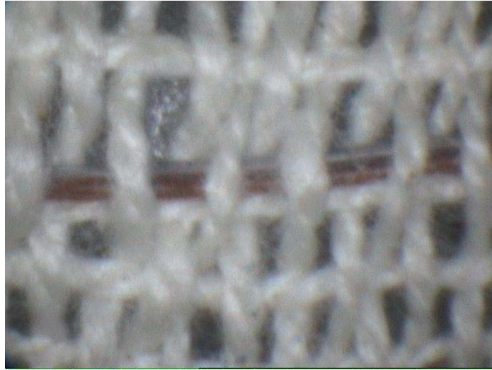
Figure 4.1: Insulated Thermocouple Woven inside Fabric
