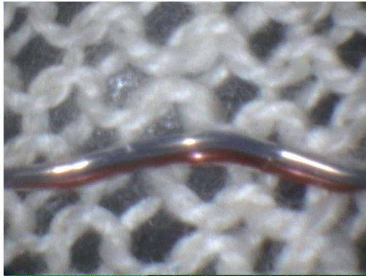
Figure 4.7: Insulated Thermocouple Interlaced into Knitted Fabric
