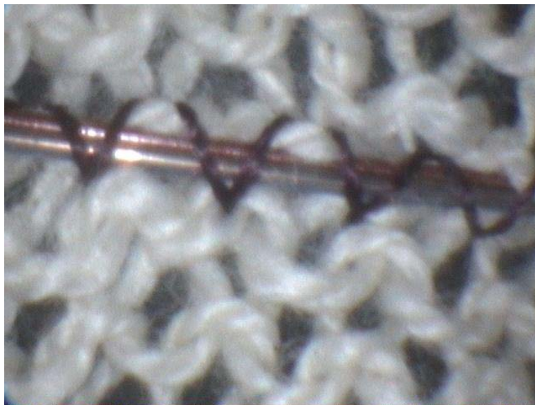
Figure 4.8: Insulated Thermocouple Stitched on Knitted Fabric
