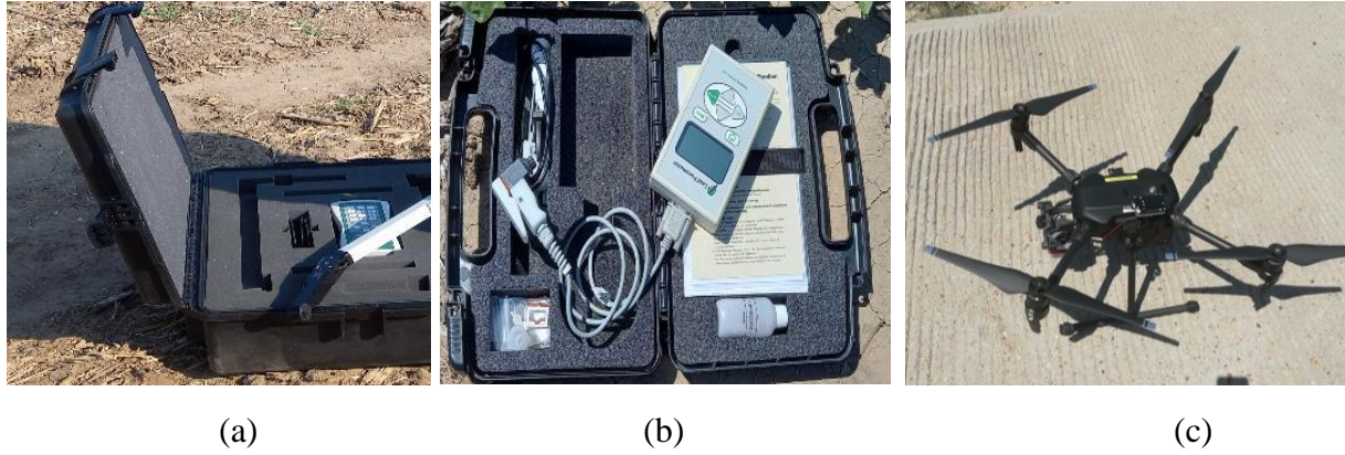
Photo 3-2 Pictures of devices used to collect data (a) LAI-2200C, (b) Porometer, (c) UAV 3.1.4 Standardized Penman-Monteith reference evapotranspiration model
