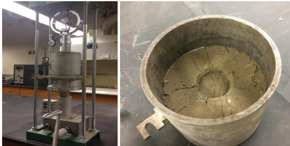
Figure 3-8 CBR test setup and a tested specimen (ASTM C157)
