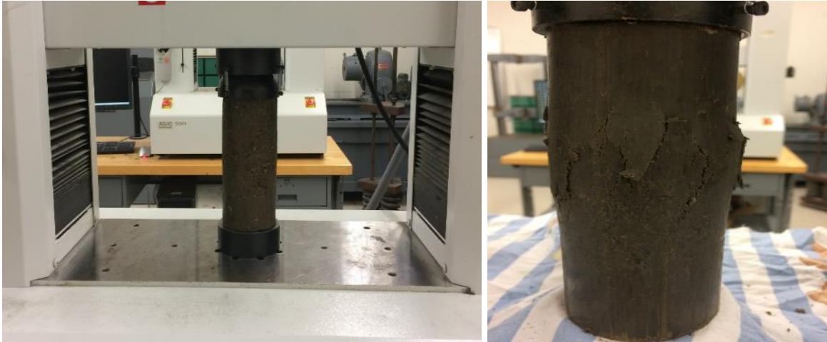
Figure 3-6 Unconfined compression test (ASTM D1633)
