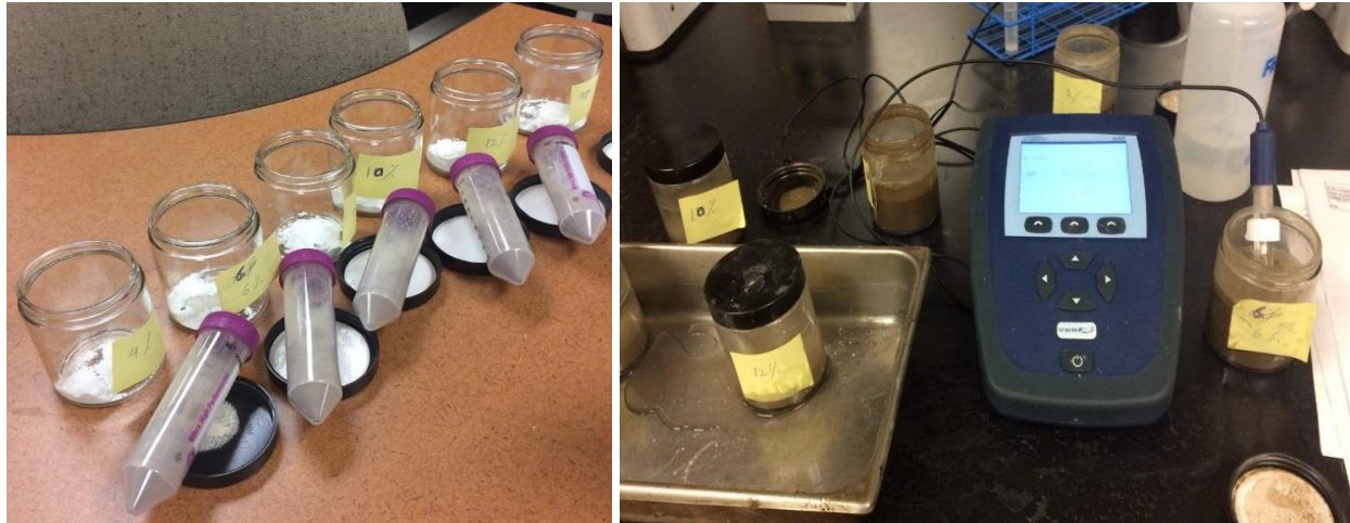
Figure 3-4 Estimation of initial lime content (ASTM D6276)
