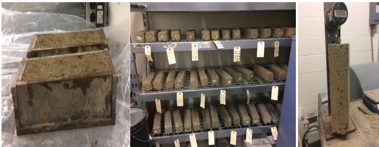
Figure 3-7 Shrinkage test setup, curing, and length measurement
