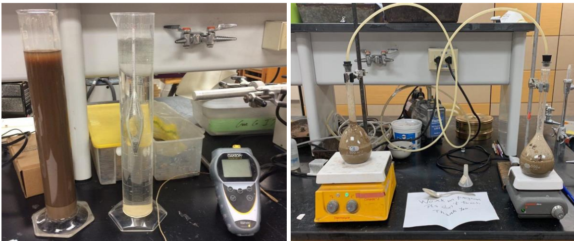
Figure 3-3 Hydrometer and specific gravity test on clay
