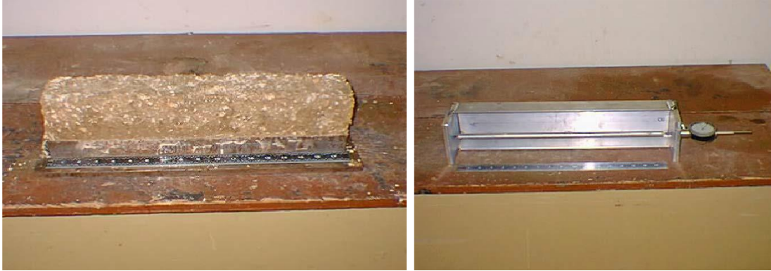
Figure 2-8 Test sample and setup for shrinkage testing (Walker 1995)
