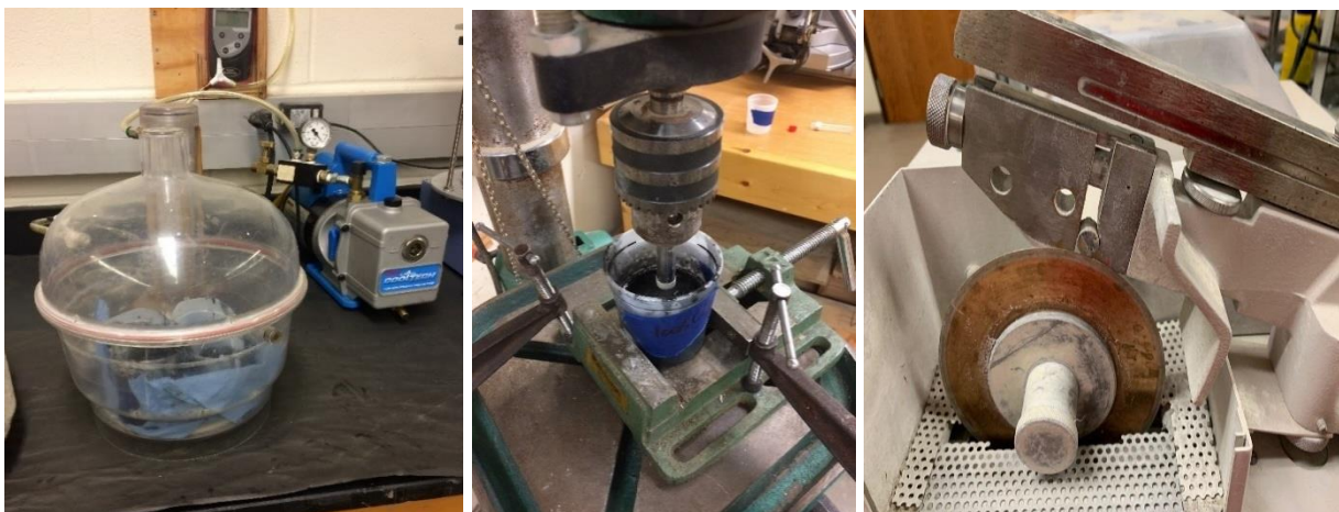
Figure 3-10 SEM sample preparation, epoxy curing, and sample coring and cutting
