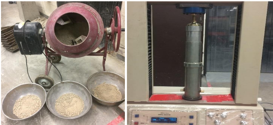
Figure 3-5 Mixing and compaction of soil-cement mixes
