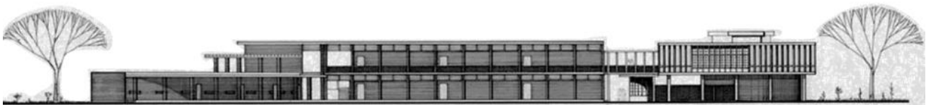
Figure 5-19 South Elevation of the Building: Shaded corridors, Verandahs, Internal Courtyards all are south facing. (Archive, n.d.)
