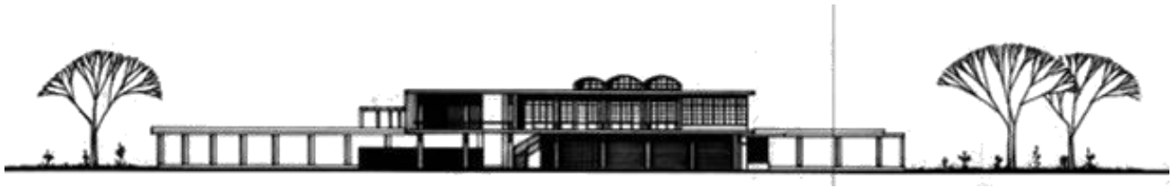
Figure 5-20 East Elevation of the Building: Architect deliberately designed the building and avoided hot summer sun on the east side. The building is elongated south to north. (Archive, n.d.)
