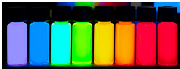
Figure 1.3 Different sized quantum dots. QDs emit different wavelengths as a function of their size (left to right = small to large diameter). Photo from Wikipedia.
