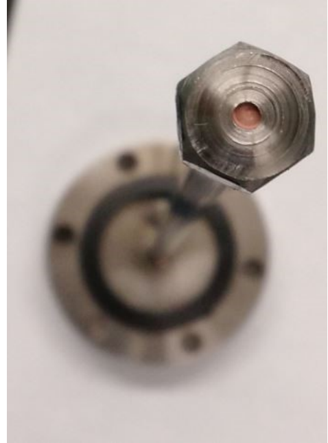
Figure 2.11 Custom TEM-grid jig to test particle beam in-vacuum. TEM grid (copper-colored) inside hole in holder.
