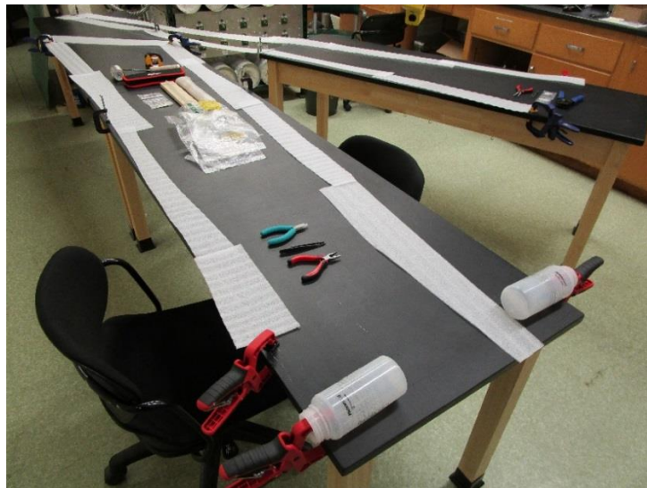
Figure 3.7: The rearranged assembly setup and how the wires are clamped down.
