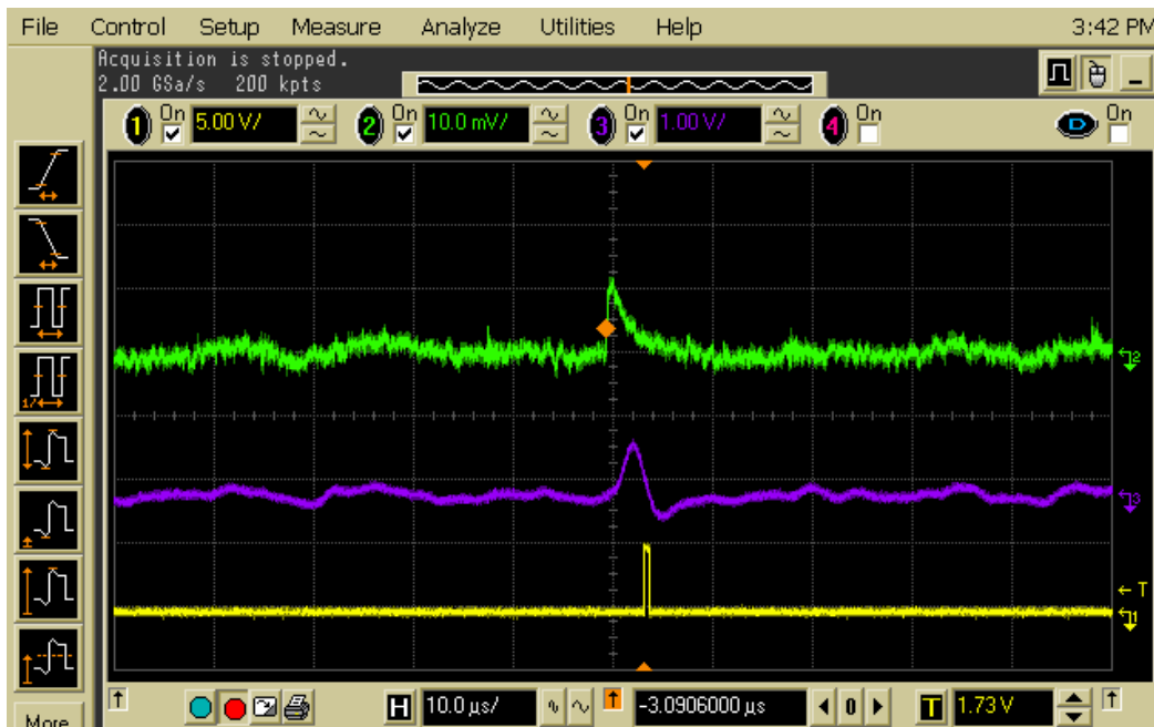
Figure 5.4: Preamplifier (green), amplifier (purple), and TTL (yellow) signal of a neutron pulse from the MPFD.
