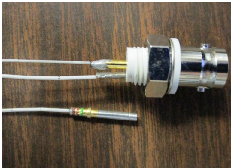
Figure 3.14: The use of acid flux solder to connect nickel wire to the pin connectors for the electrical feed-through (bottom) and BNC connectors (top).
