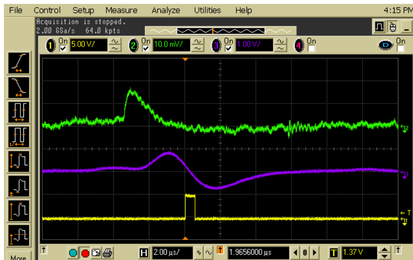
Figure 5.3: Discharges caused by nickel shavings.
