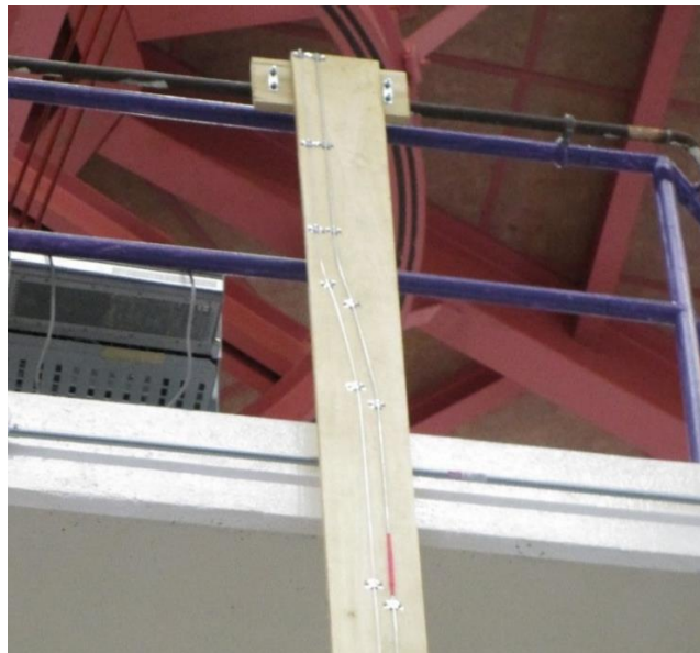
Figure 4.2: The completed mock-up mounted to the thermal column at the KSU TRIGA MARK II nuclear reactor.
