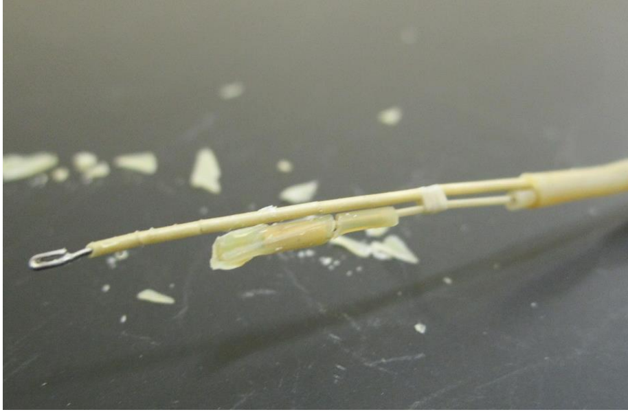
Figure 5.12: The post bake of a MPFD array at 600°F after 24 hours and the results of the damage caused by both radiation and high temperatures.
