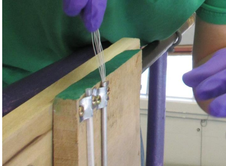
Figure 4.3: Shown is the method for inserting the MPFD array into the flux wire port.
