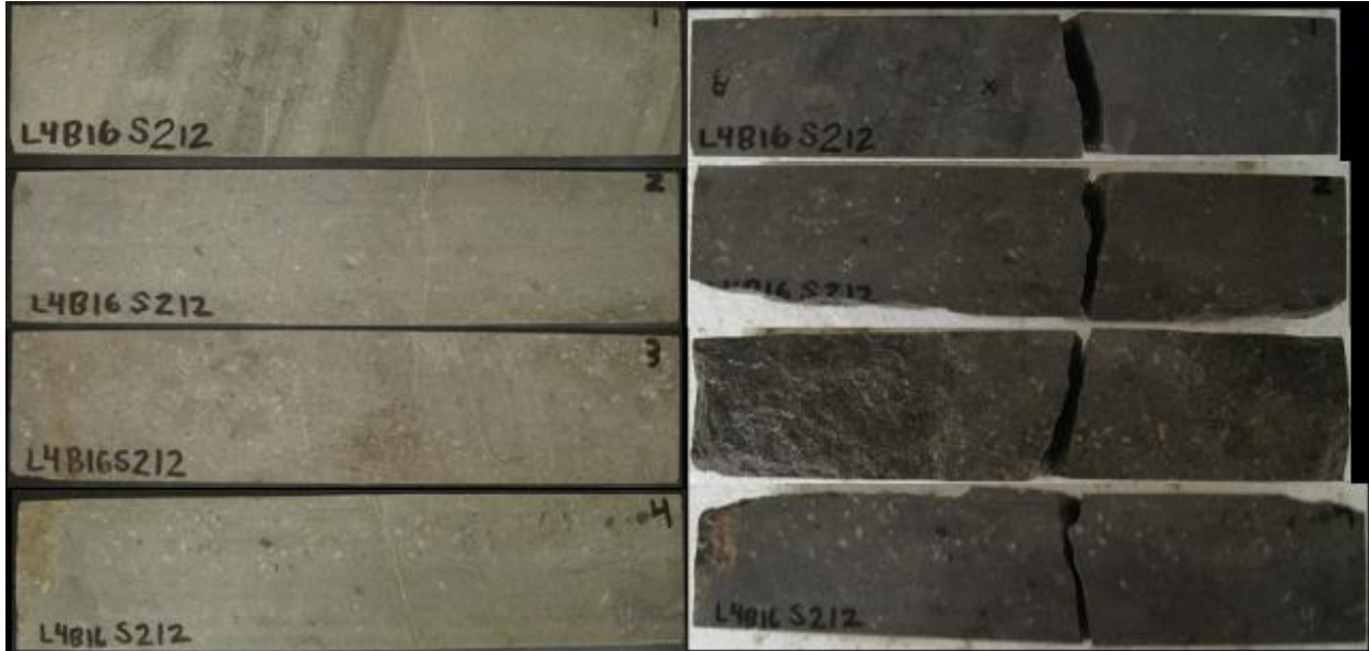
Figure 5.23: L4 Sample 212 After Salt-Frost Exposure
