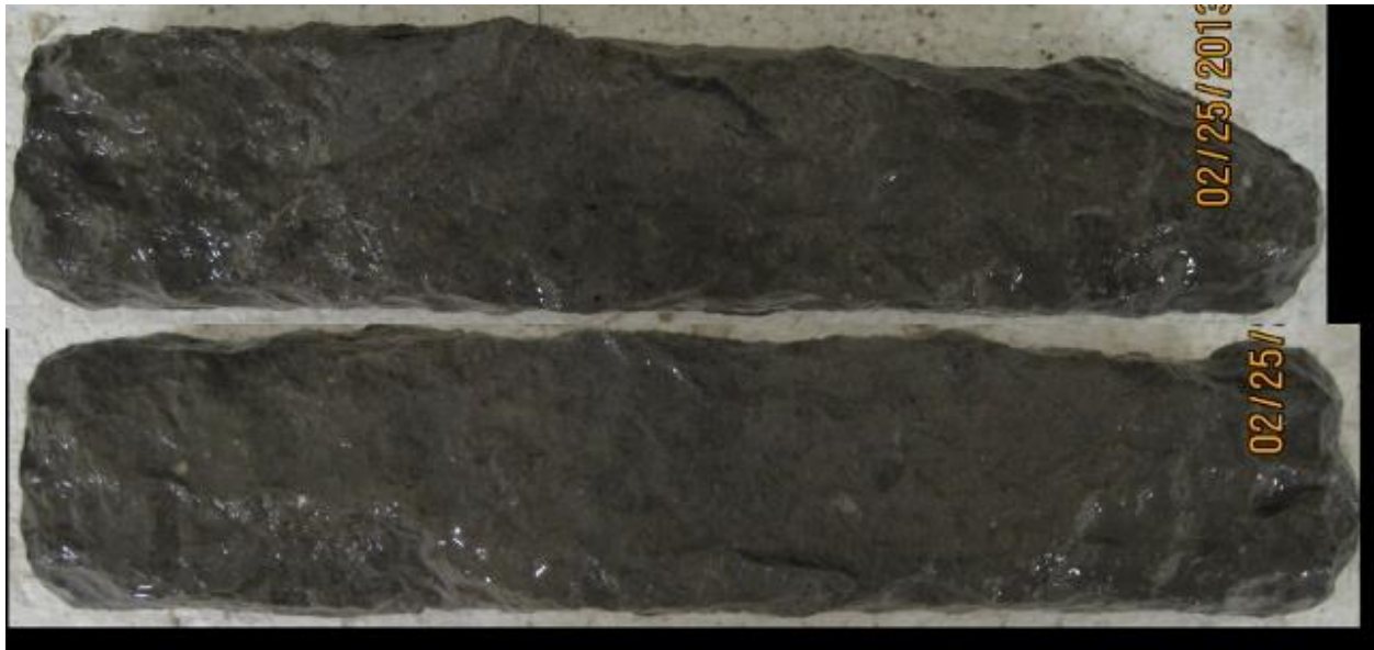
Figure 5.17: Unidentifiable Prism After Salt-Frost Exposure
