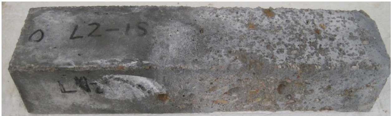
Figure 5.32: L2 Half-Immersed Concrete Prism
