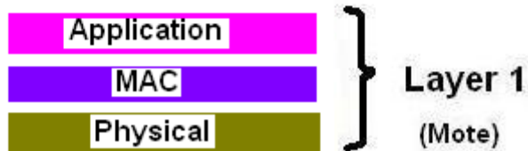
Figure 2.2 Network Protocol Architecture showing Layer 1 and Layer 2
