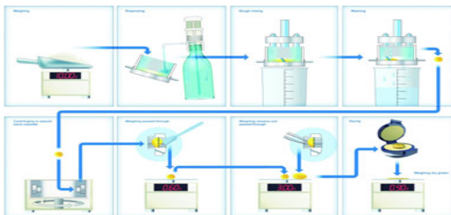
Figure 1.4 Schematic diagram of Glutomatic washing system (Accessed from http://www.perten.com/pages/ProductPage418.aspx?epslanguage=EN ).
