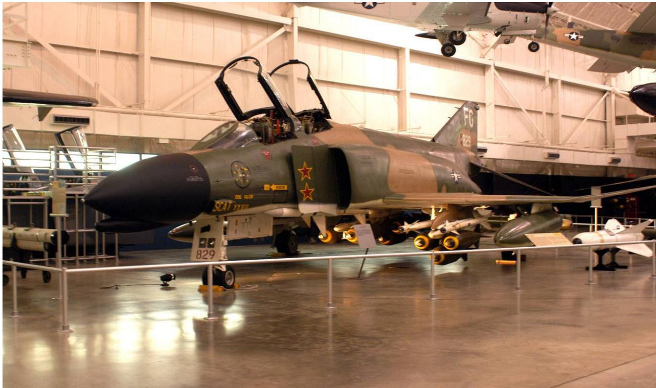
**Figure B.14 F-4C configured for multi-role mission. This was the usual configuration for *Phantoms* tasked with an air-to-ground primary mission followed by a secondary air-to-air encounter. This particular F-4C was Colonel Olds' mount during Operation Bolo.<sup>14</sup>**
