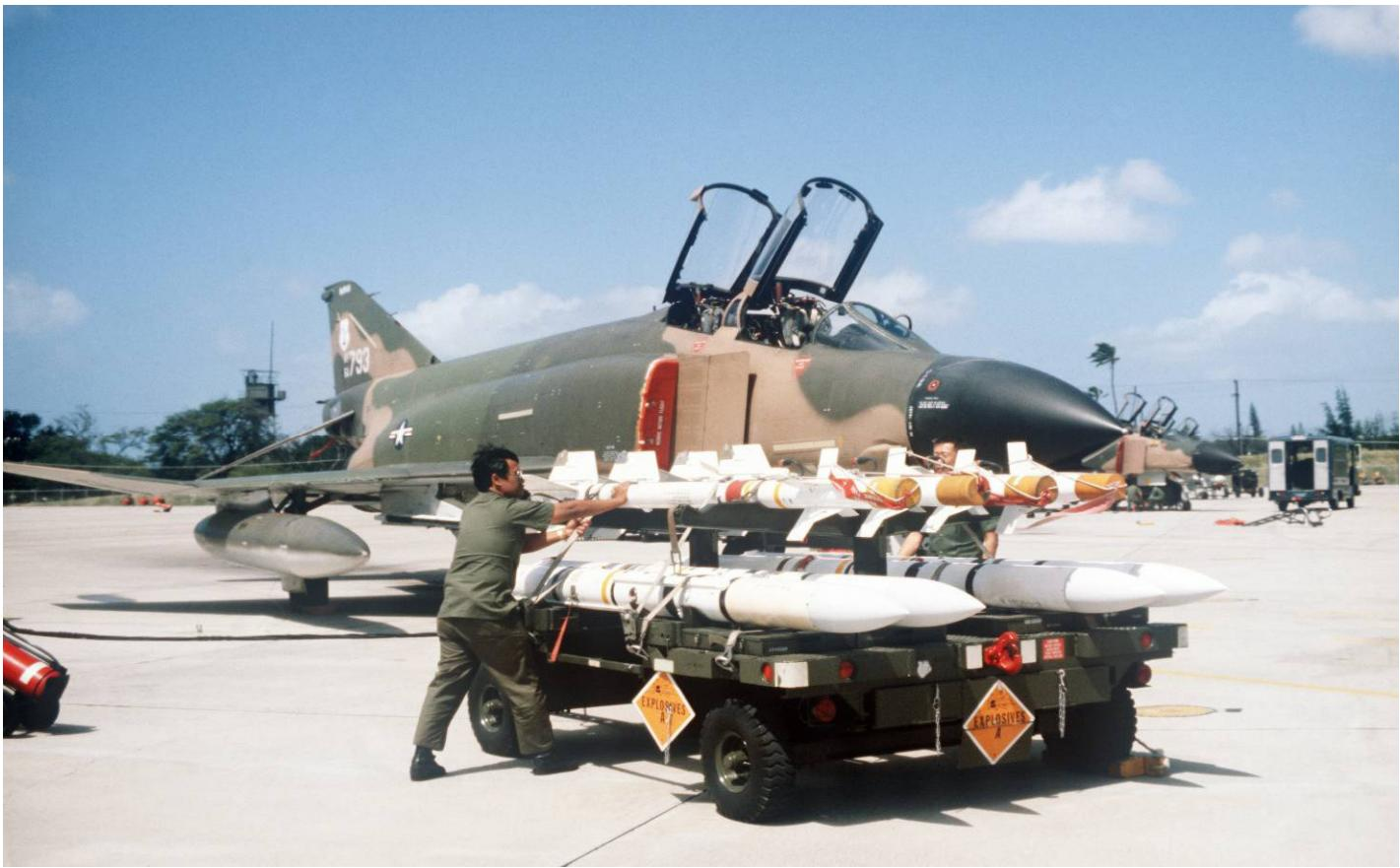
**Figure B.13 AIM-9 *Sidewinders* (top row) and AIM-7 *Sparrows* (bottom row) being loaded on an F-4C. Note crewman for scale.<sup>13</sup>**
