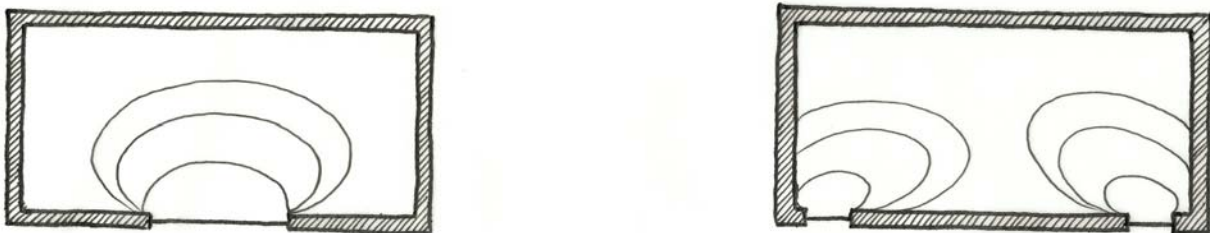
Figure20d. These plans, with contours of equal illumination, illustrate how light distribution is improved by admitting daylight from more than one point. (Drawn by author, adapted from Heating, Cooling, Lighting , p. 322)
