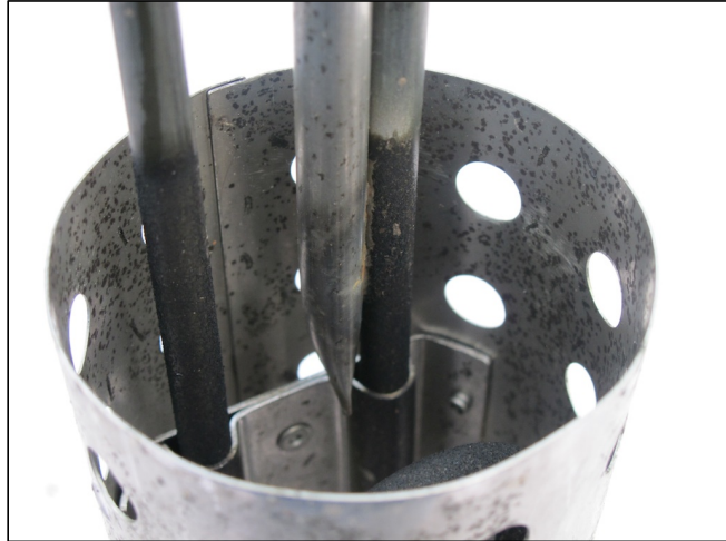
Figure 4.9 Primary Study Bucket Heater and Galvanic Corrosion
