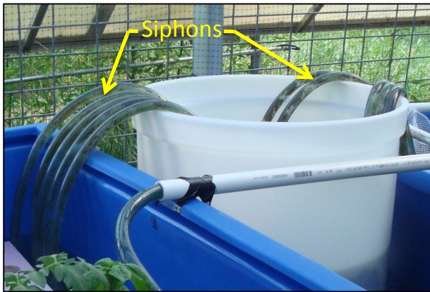
Figure 4.23 Water Circulation: Pilot Study Siphons vs. Proposed Facility Gravity Weir Flow
