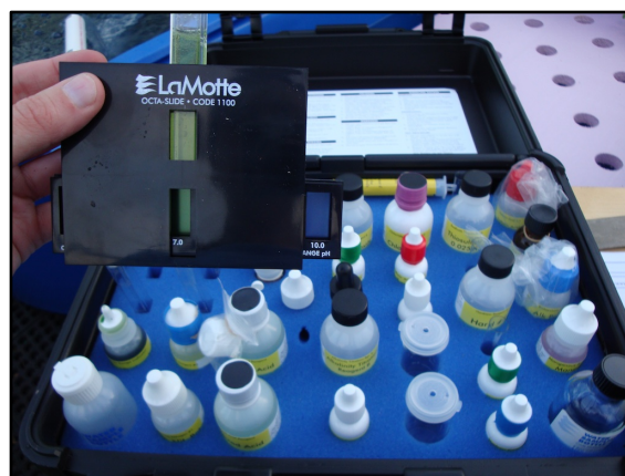
Drop test kit utilized to monitor water quality in our Kansas facility
