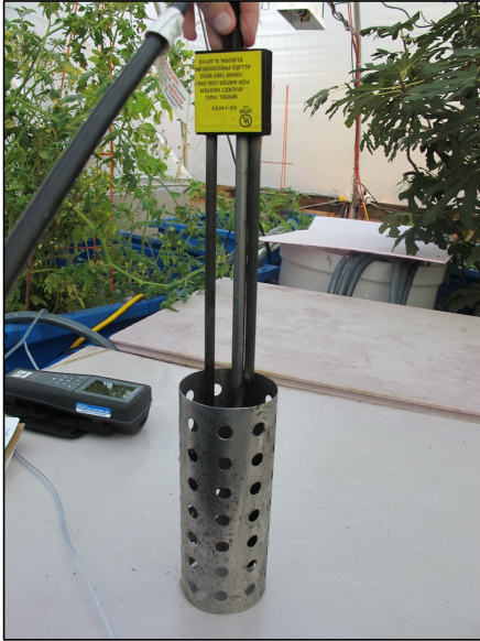
Figure 4.9 Primary Study Bucket Heater and Galvanic Corrosion
