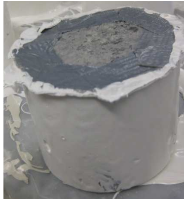
Figure A.1 - Three inch concrete specimen with protective duck tape
