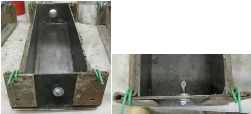
Figure 3.2 - Freeze thaw mold and stainless steel pin setup
