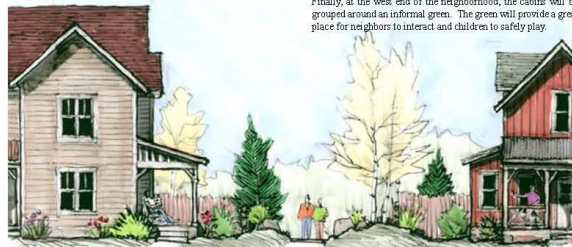
The mid-block pedestrian trail fits into a generous 20 foot wide Right-of-Way. Low fences, gentle earth mounds, and privacy fences in places create a diversity along the path. Homes along either side can be placed so that the side porches orient toward the trail, encouraging neighborly interaction.
