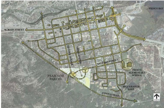
Above is an aerial showing the Peak One Parcel in its context. Resolving the street grid by means of two "T" intersections and a loop is the guiding principle for this street geometry.
