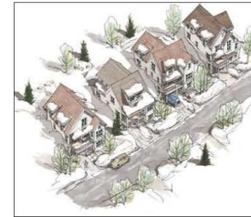
The right-of-way has adequate space on each side for snow storage, but garages are located relatively close to the street to reduce the amount of snow-shedding required. Clearance porches along the fronts of homes create habitable space along the building edge and welcoming faces to the street.
