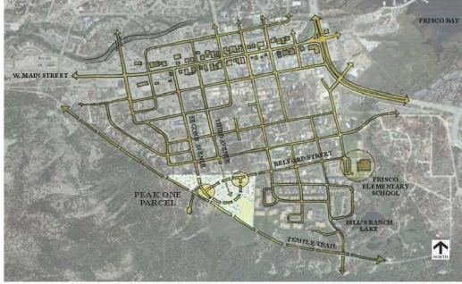
Above is an aerial showing the Peak One Parcel in its context. Resolving the street grid by means of two "T" intersections and a loop is the guiding principle for this street geometry.
