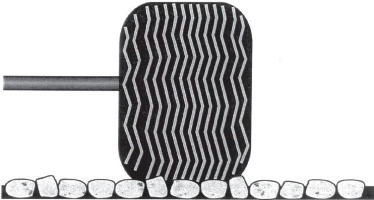
Figure 2.11 Chip Seal with Cubical Aggregates (Wood et al. 2006)
