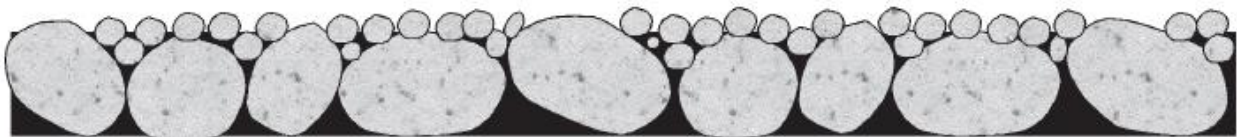
Figure 2.3 Racked-In Seal (Wood et al. 2006)
