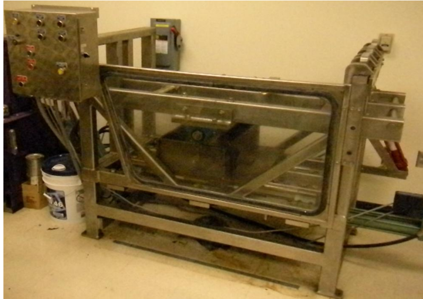
Figure 3.5 PMW Compactor Machine
