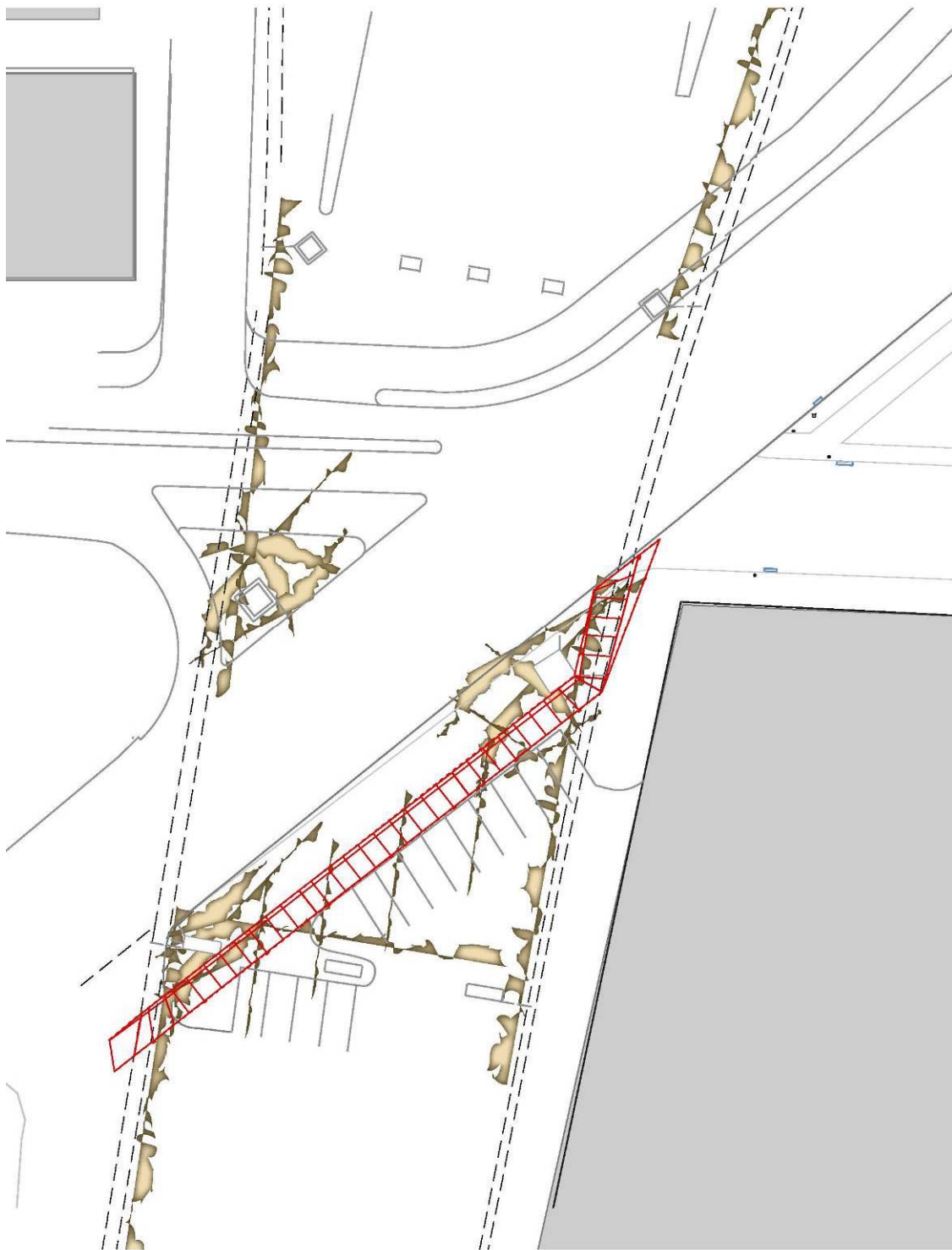
Figure 5.2. Pigeon droppings pattern and proposed canopy location.
