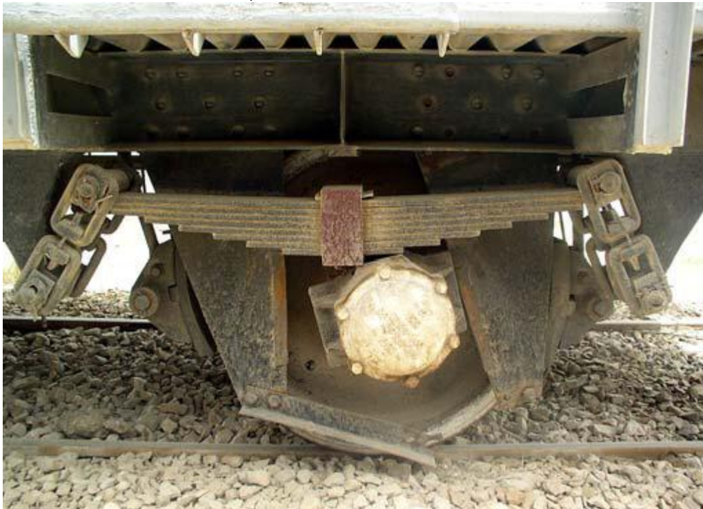
Reconstruction teams are often charged with organizing the repair of equipment, such as this train axle which is missing the brake block, oil feed, and axle cover. Source: Bechtel Corporation, 2003.
