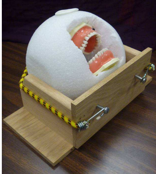
Figure 4-9. Replicated Human Head with Typodont
