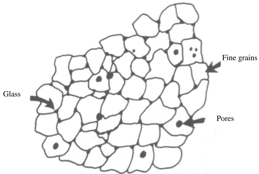
Figure 4.2 The microstructure of a typical dense ceramic (Lee and Rainforth, 1994)
