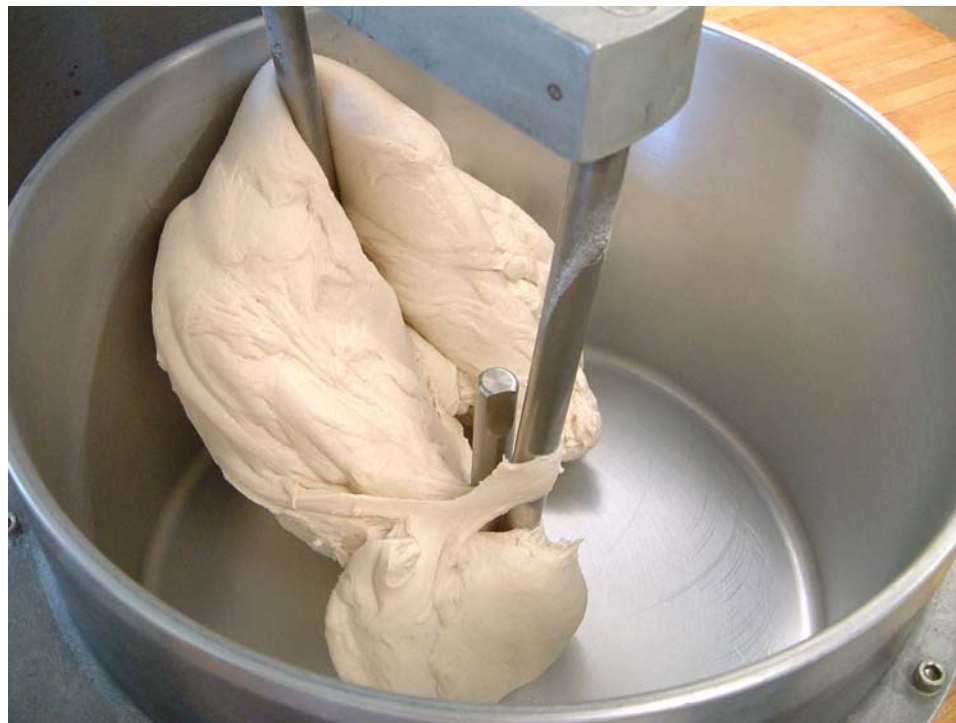
Figure A.2. Water bath & Mixer. Mixing bowl temperature maintained at 6 °C by a circulating refrigerated water bath.
