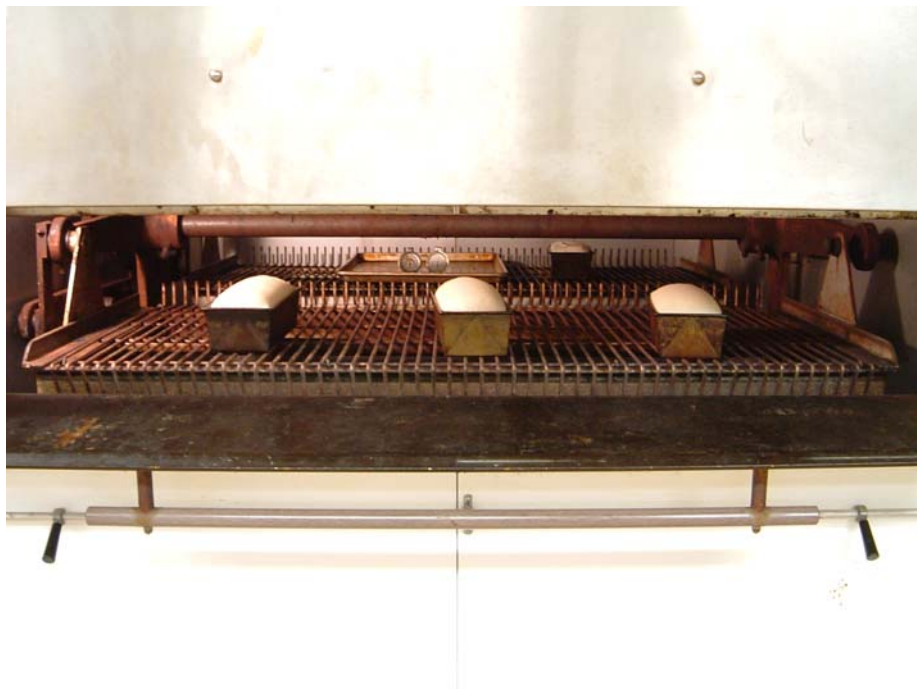
Figure A.19 Baking. The doughs were baked for 22 minutes at 210°C (410°F) in a reel oven.
