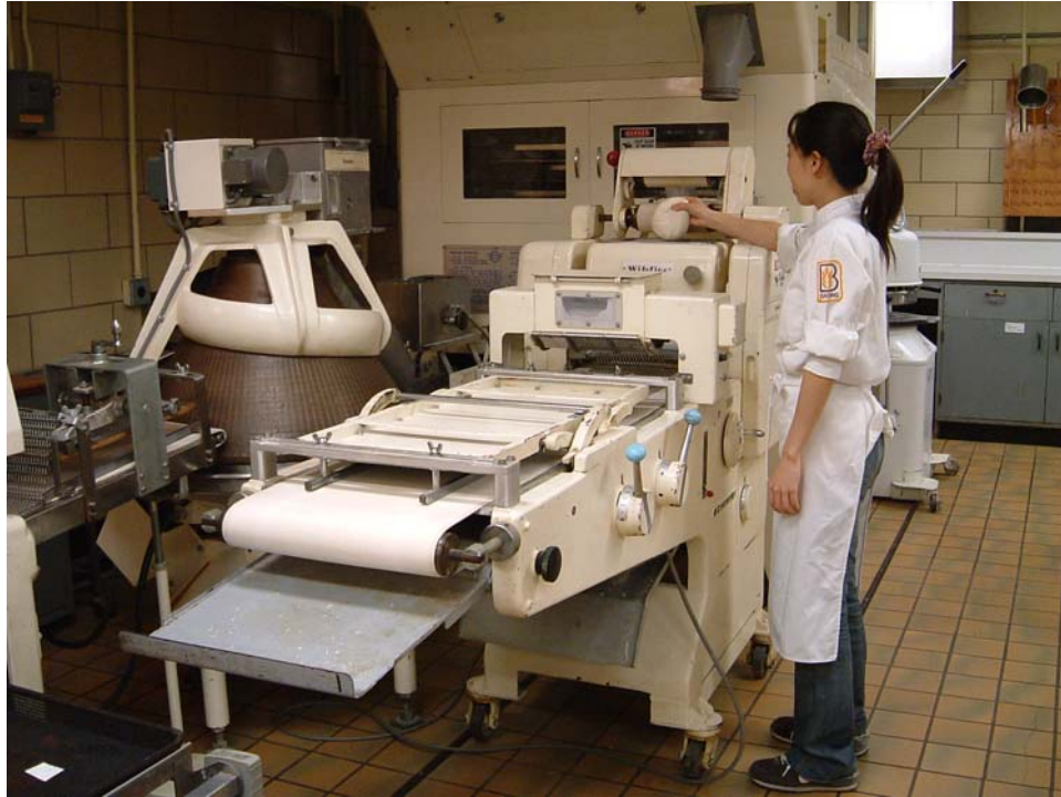
Figure A.8 Sheeter/ Molder. After 5 minutes floor time, each dough piece was sheeted and molded by the Oshikiri equipment.
