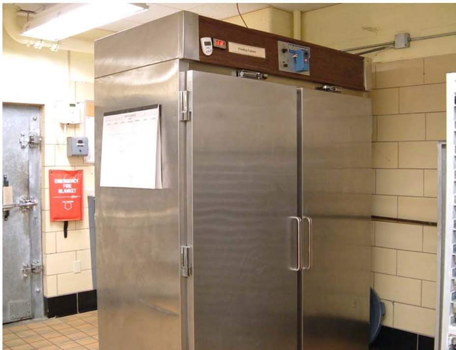
Figure A.16 Proofing Cabinet. Doughs were proofed in proofing cabinet at 40°C (104°F) and 70% humidity.
