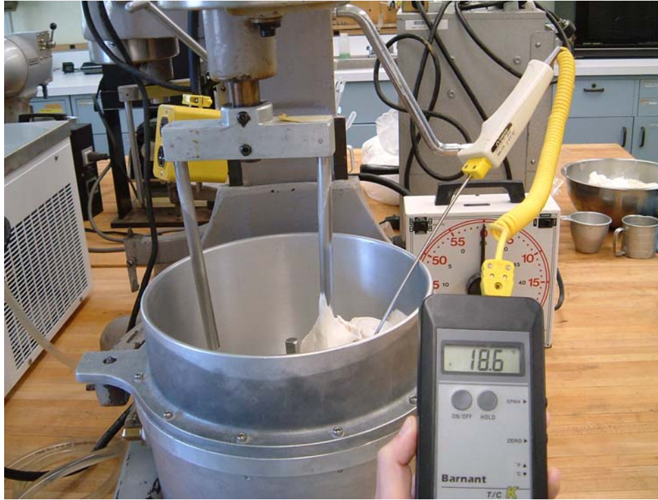
Figure A.4 Dough temperature measured after mixing in mixing bowl.
