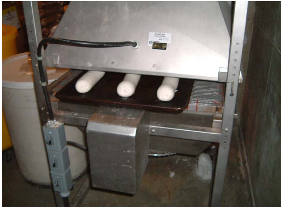
Figure A.10 Air impingement blast freezer operating at -20 °C.
