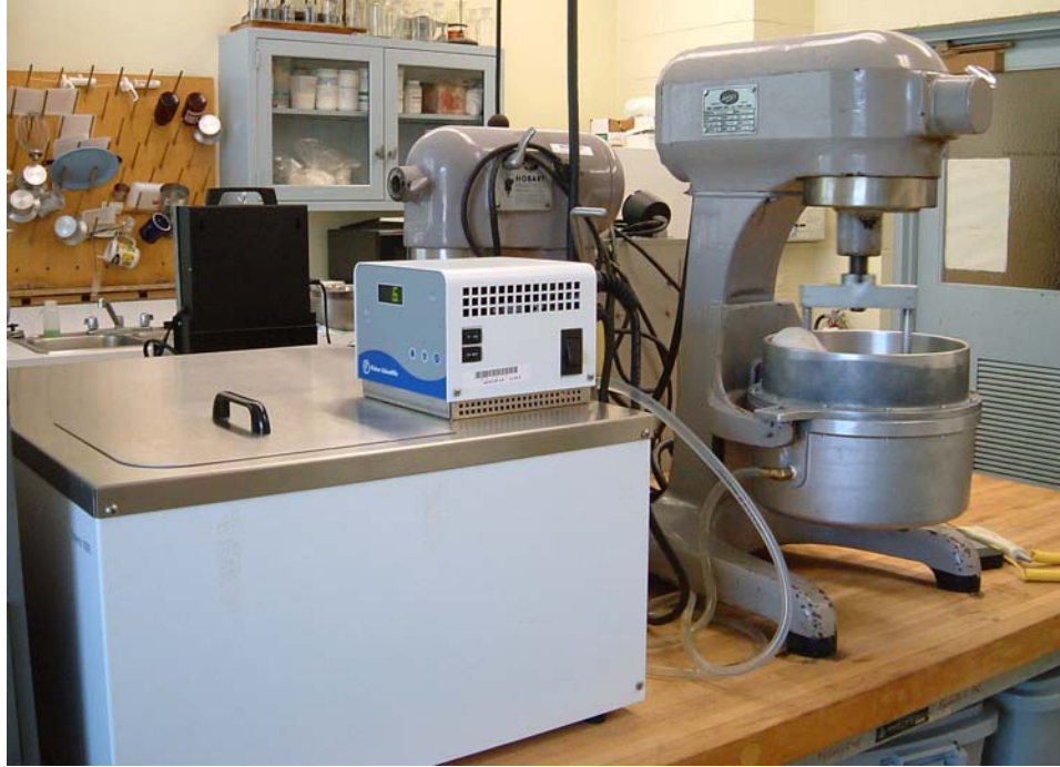
Figure A.2. Water bath & Mixer. Mixing bowl temperature maintained at 6 °C by a circulating refrigerated water bath.
