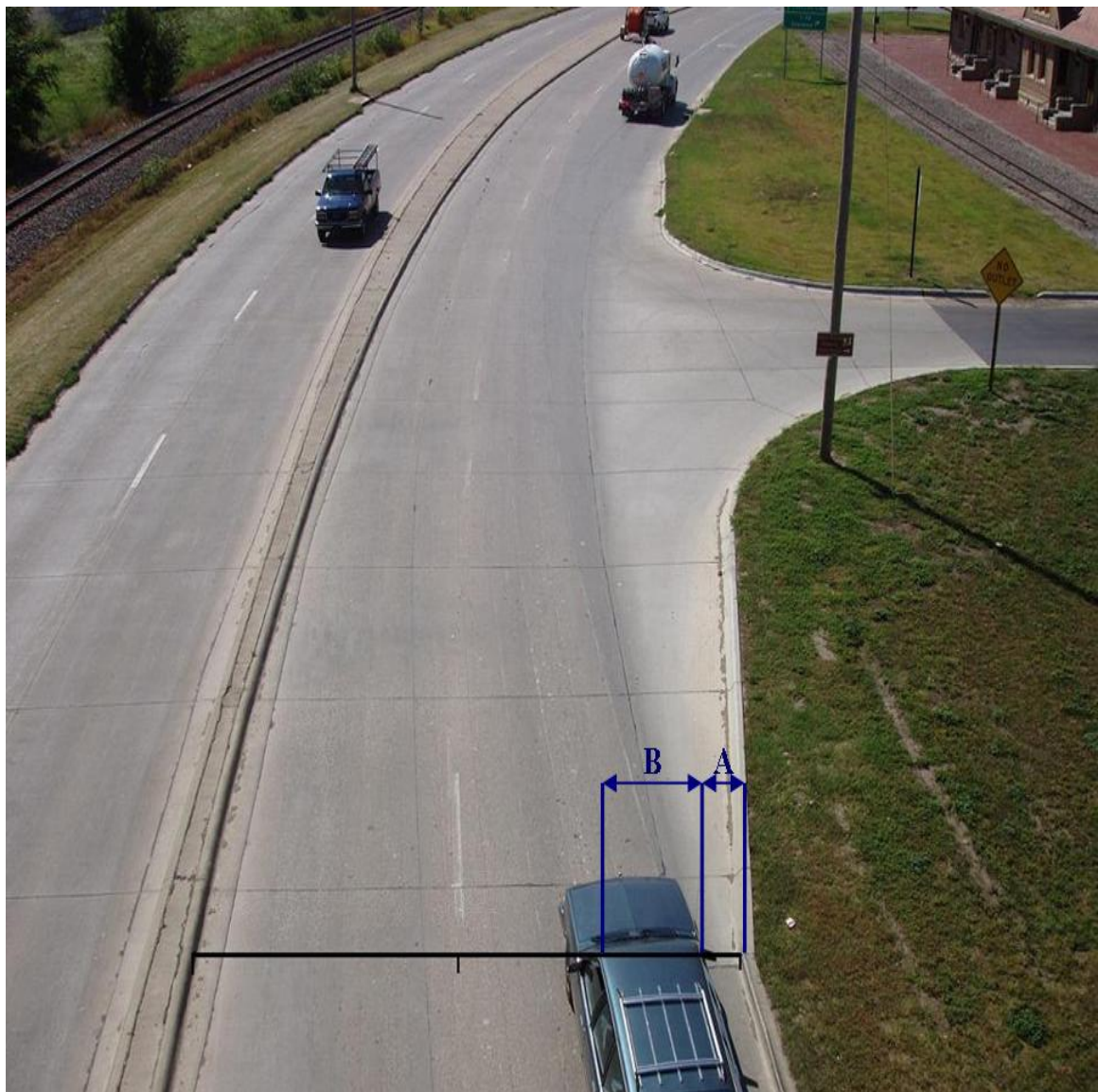
Figure 3-6 Picture Showing the Measurement of Distance on the Television Screen
