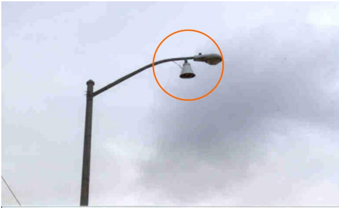
Figure 3-3 Camera with a Fish-Eye Lens Setup on a Utility Pole at Test Site (First Stage)
