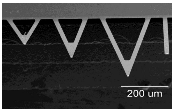
Fig 1.3 Cantilevers. Adapted from www.mobot.org . The top surface of a cantilever (the surface opposite to the probe side) is often coated with a thin film of gold or aluminum to maximize the reflected light intensity.
