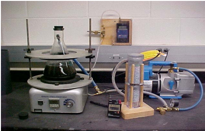
(c) Loose mixture preparation
