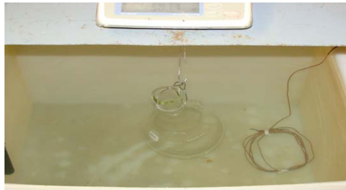
(g) Mass of flask in water
