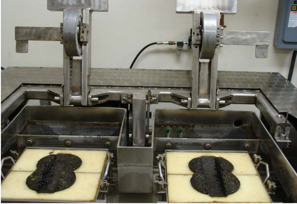
Figure 3-9 Finally Failed Specimens by HWTD
