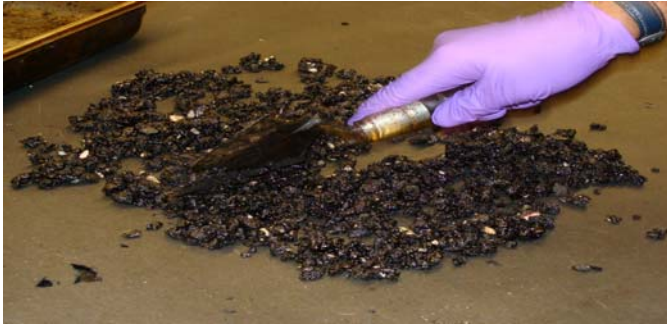
(c) Loose mixture preparation
