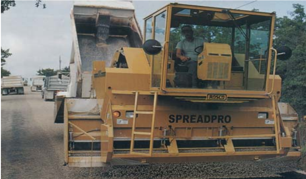
Figure 2-13 Self-Propelled Chip Spreader (Caltrans Division of Maintenance, 2003)
