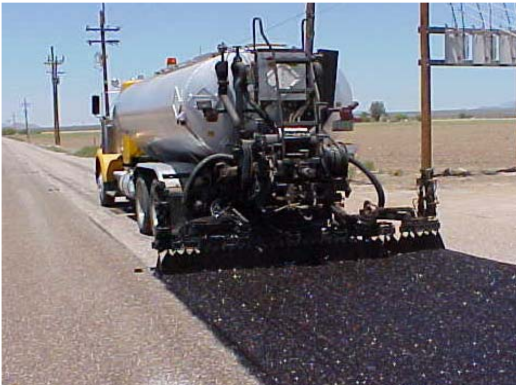
Figure 2-12 Asphalt Distributor (Caltrans Division of Maintenance, 2003)
