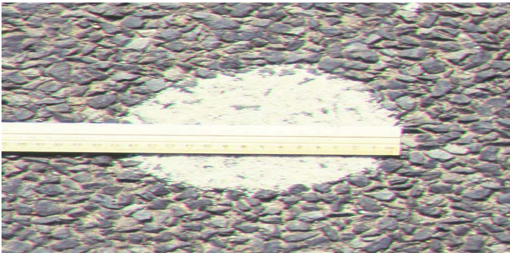
Figure 2-15 Sand Patch Test (Caltrans Division of Maintenance, 2003)
