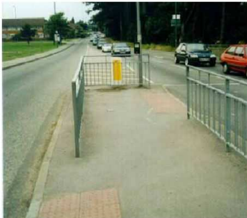
Figure 1.7: Staggered Crosswalk with Fencing
